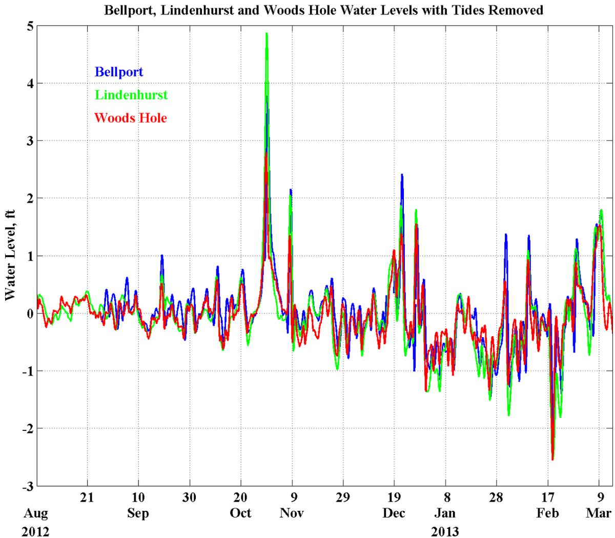
**Figure 6, Times series of water levels from Bellport, Lindenhurst and Woods Hole, MA with the tides removed showing the high degree of similarity along ~300 km of coastline and within Great South Bay.**
