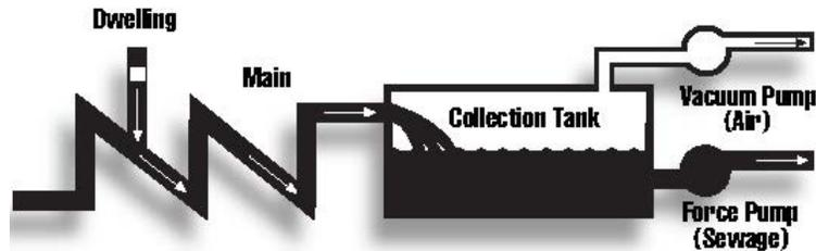
The pipe is designed to follow the contour of the land where the ground slopes naturally, and is most economical in flat terrain. Small lifts in the pipe may be used when necessary to keep excavation shallow. At the pumping station, the mains empty into a collection tank. The wastewater is then treated nearby or pumped to another location for treatment.
