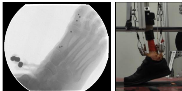
Figure 1. A screenshot of an X-ray frame (left) of a cadaver while mounted to the custom rig (right). Beads are shown as six black circles on the first metatarsal and phalanx.
