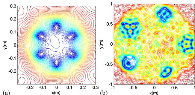
Figure 2. The LSM contours corresponding to different values of  $\log\|g_z^\alpha\|$  for (a) the star shaped target and (b) the five objects target.
