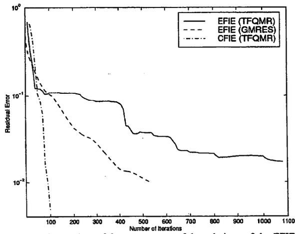
Figure 3. Comparison of the convergence of the solutions of the EFIE using TFQMR (solid line), EFIE using GMRES (dotted line), and CFIE with  $\alpha = 0.5$  using TFQMR (dashed line) for a perfectly conducting rough surface.
