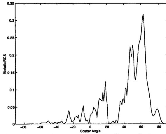
Figure 2. The vertically cross-polarized RCS of one realization versus the scatter angle  $\theta' \cos\phi'$ .
