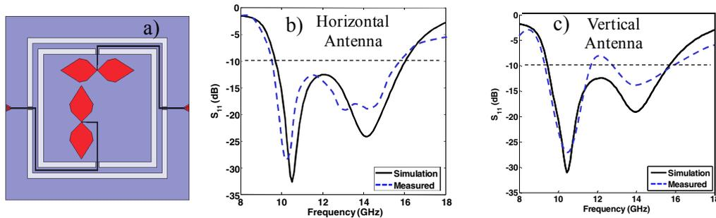
Fig. 3. a) The geometry simulated in HFSS along with the measured and simulated  $S_{11}$  for the b) horizontal antenna and c) vertical antenna
