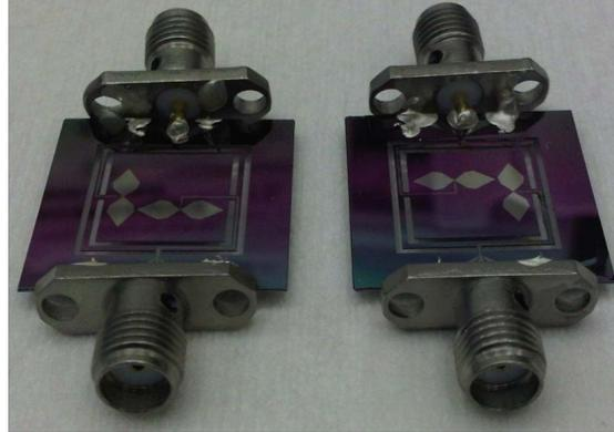
Fig. 2. Picture of finalized MEMS antennas with SMA connectors
