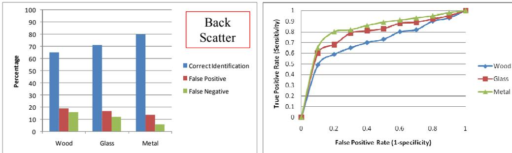
Fig. 4. a) Artificial neural network results for backscattered data for each of the target types and b) the ROC curve for the backscattered data
