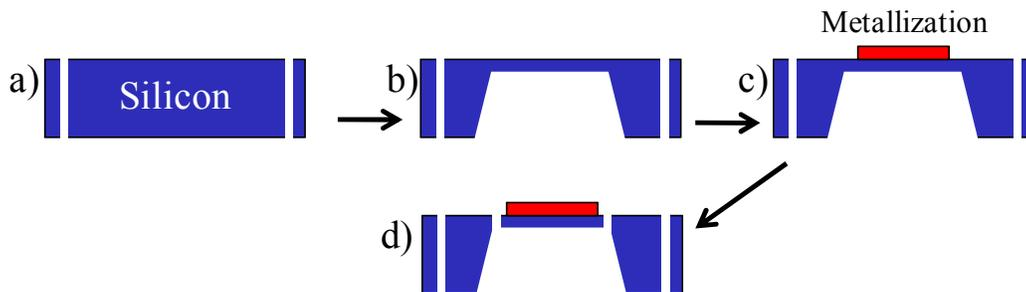
Fig. 1. Processing flowchart showing a) through-silicon vias b) backside cavity etch c) antenna metallization and d) platform release
