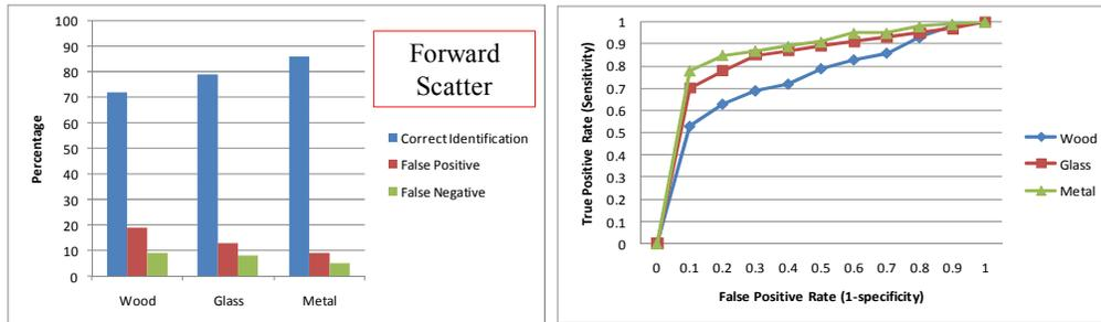
Fig. 5. a) Artificial neural network results for forward scattered data for each of the target types and b) the ROC curve for the forward scattered data
