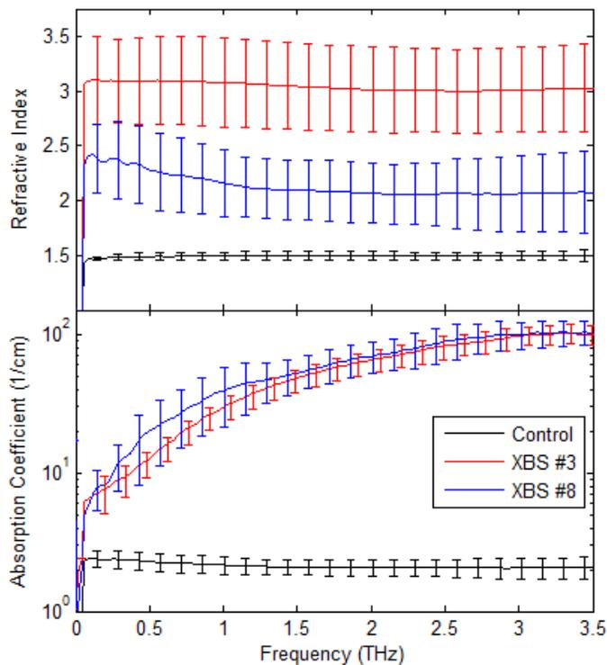
Fig. 1. Refractive index (top) and absorption coefficient (bottom) THz spectroscopy results for the three different coatings. Error bars illustrate standard deviations in the 8 separate measurements taken on each sample.
