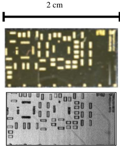
Fig. 2. Photograph of microchip without XBS coating (top) and frequency domain THz image of the same chip without XBS coating, taken at 3 THz and 50  $\mu\text{m}$  pixel size.
