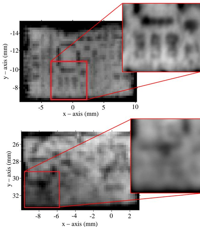
Fig. 3. THz time-domain image of microchip with 345  $\mu\text{m}$  (top) and 1500  $\mu\text{m}$  (bottom) of the control coating with 250  $\mu\text{m}$  pixel size. Inset illustrates a reduced section of the sample with a 50  $\mu\text{m}$  pixel size.
