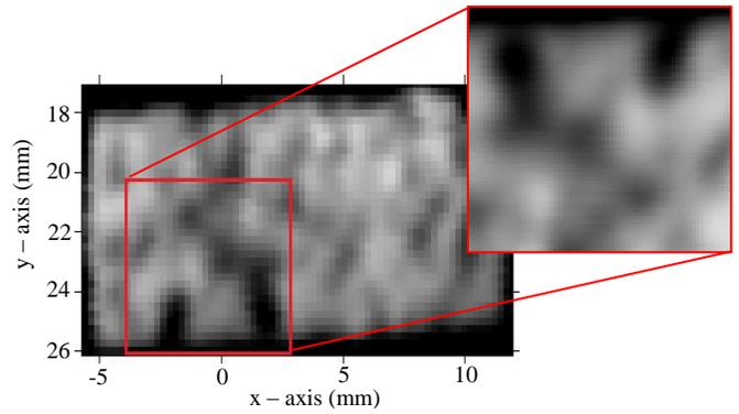
Fig. 4. THz time-domain image of microchip with 650  $\mu\text{m}$  of the XBS #3 coating with 250  $\mu\text{m}$  pixel size. Inset illustrates a reduced section of the sample with a 50  $\mu\text{m}$  pixel size.
