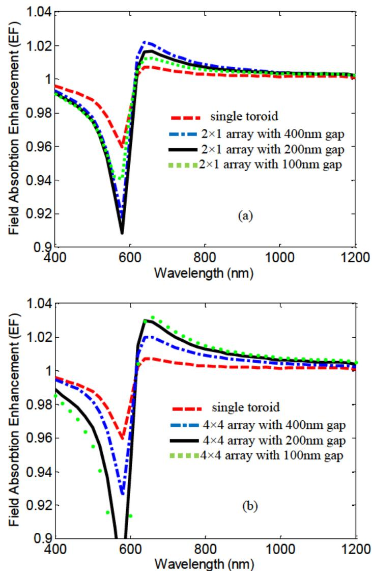
Fig. 3. MoM field enhancement factor (EF) in silicon, due to a (a)  $2 \times 1$  nanotoroid array and (b)  $4 \times 4$  array with separation gaps of  $400\text{ nm}$ ,  $200\text{ nm}$ ,
