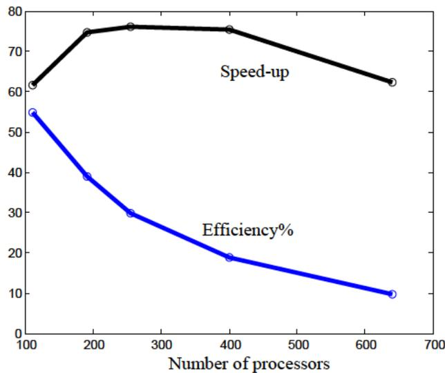
Fig. 2. Speed-up and efficiency of field enhancement computation at wavelength of 610 nm for a 2x1 nanotoroid array of Figure 1.
