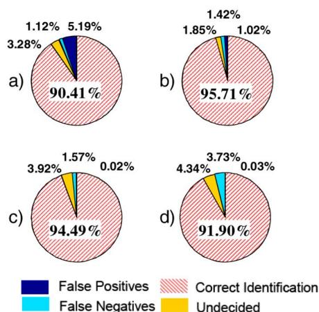
Fig. 4. Results using a double cutoff of 0.4 and 0.7 with a testing set of noise  $\sigma_n = 0.1$  and a training set of (a) no noise, (b)  $\sigma_n = 0.1$ , (c)  $\sigma_n = 0.2$ , and (d)  $\sigma_n = 0.3$ .
