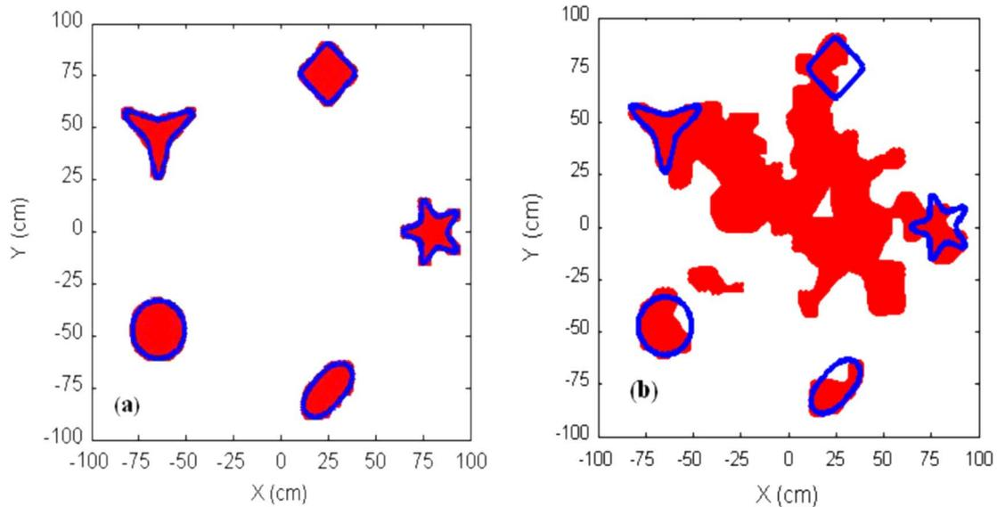
Fig. 5. Final reconstruction of a five cylinders after 12 555 iterations at 3 GHz (a) using configuration of (3); (b) full measurement configuration.
