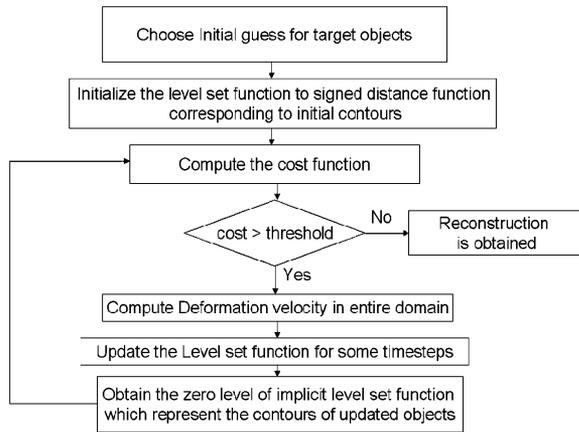
Fig. 1. The level set shape reconstruction algorithm.
