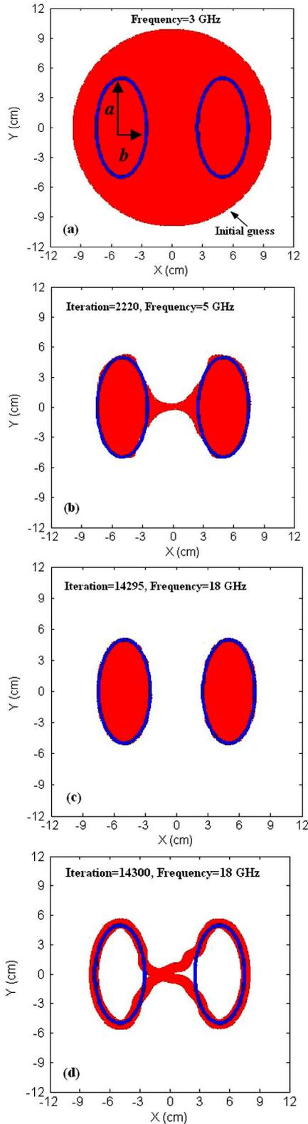
Fig. 3. Reconstruction of two elliptical cylinders: (a) initial guess, (b) after 2220 iterations using full-band scheme, (c) after 14295 iterations using full-band scheme, and (d) after 14300 using narrowband scheme.
