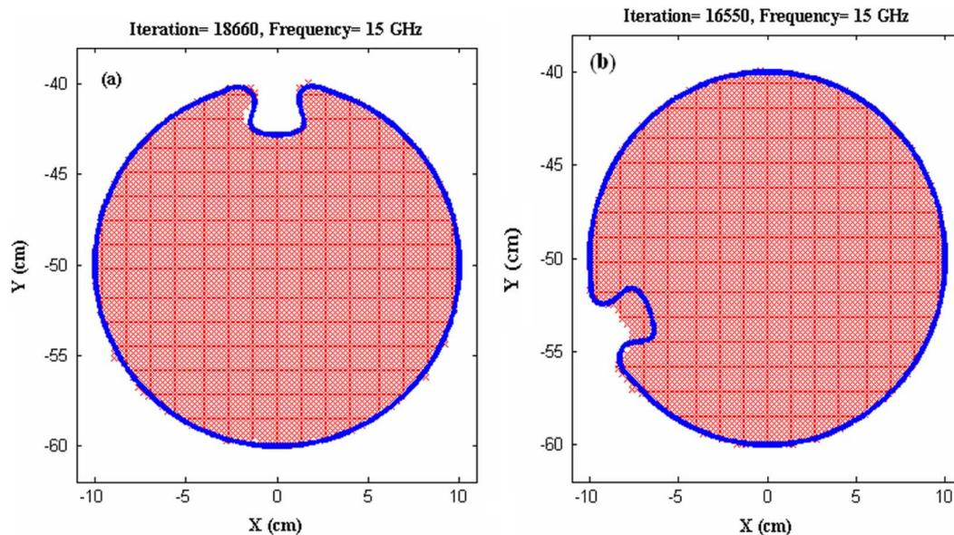
Fig. 8. Crack position in a cylinder at (a) top and (b) oblique.
