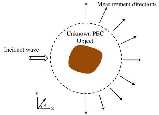
Fig. 2. Proposed incident and measurement configuration.
