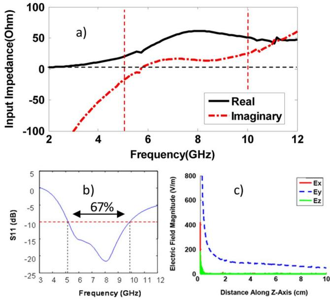
Fig. 2. (a) The input impedance and reactance of the antenna in air (b) the simulated  $S_{11}$  of the antenna referenced to  $50 \Omega$  in air and (c) the magnitude of the electric fields as a function of distance from the antenna when the  $y$ -directed port is excited (port  $e'e$ ) in air.
