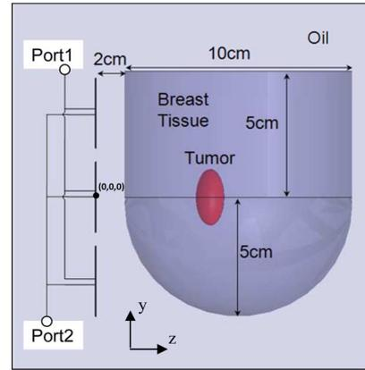
Fig. 4. The breast model with ellipsoidal tumor utilizing a three element array.
