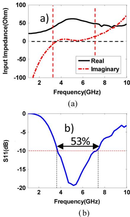
Fig. 3. (a) The simulated  $S_{11}$  of the antenna in oil and (b) the input impedance and reactance of the antenna in oil.
