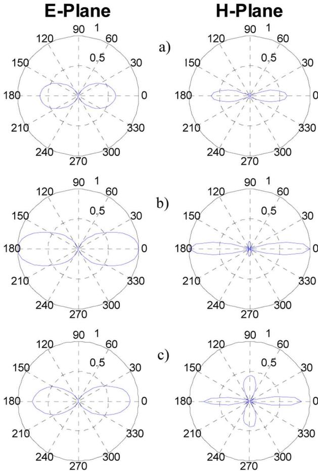
Fig. 6. Array radiation patterns at (a) 4 GHz (b) 5.5 GHz and (c) 7 GHz.
