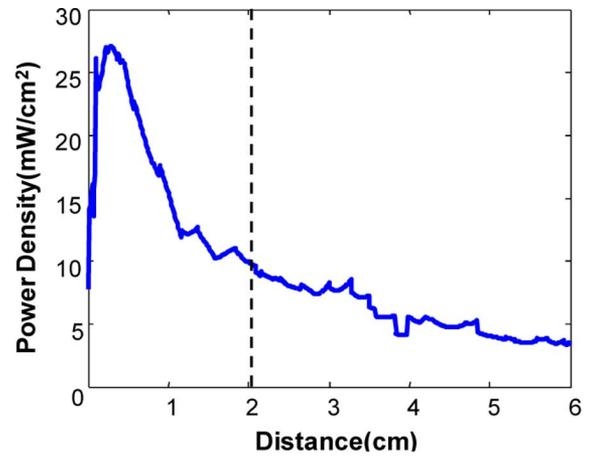
Fig. 5. Power density as a function of distance from the antenna array immersed in oil along the main beam.
