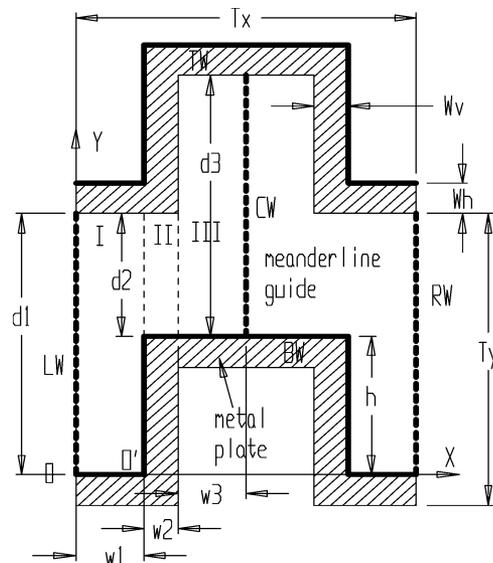
Fig. 1. Unit cell of a meanderline polarizer.
