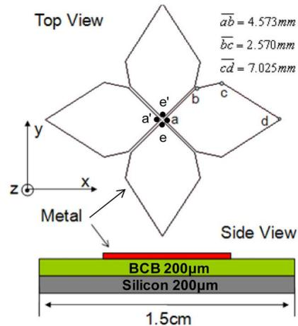
Fig. 1. Geometry of designed Fourtear antenna.
