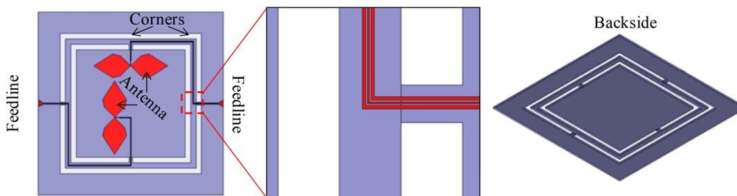
Fig. 1. MEMS Antenna design shown from the a) top view b) zoomed on the outer hinge and c) platform without antenna.
