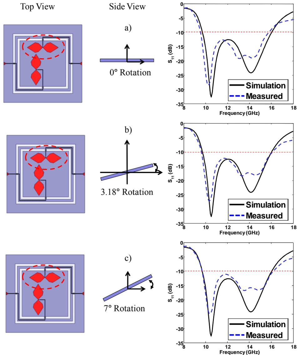
Fig. 4. Top and side views of the HFSS model and the measured and simulated  $S_{11}$  of the antenna with a)  $0^\circ$  rotation b)  $3.18^\circ$  rotation and c)  $7^\circ$  rotation.
