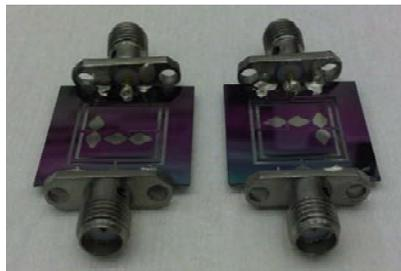
Fig. 3. Photo of two final devices ready for testing after the SMA connectors are attached using H20E epoxy.
