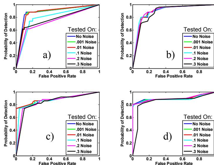
Figure 3: The probability of detection vs. the false positive rates for training on a) No Noise, b)  $\sigma_n = 0.1$ , c)  $\sigma_n = 0.2$ , and d)  $\sigma_n = 0.3$ .
