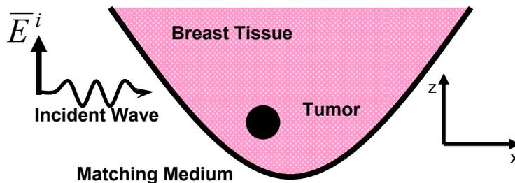
Figure 2: Model of the breast and incident plane wave at 6GHz with tumor of radius 5mm.
