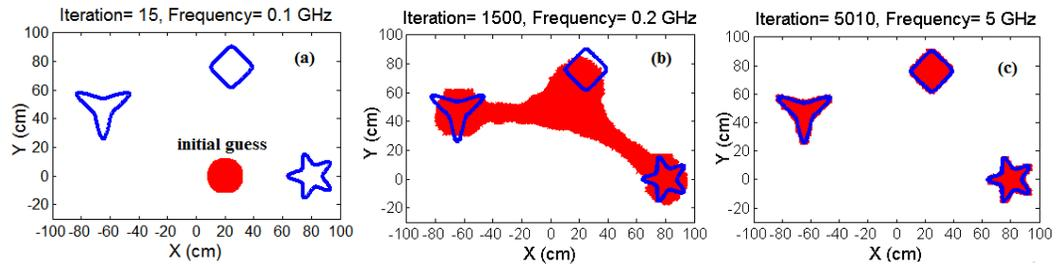
Fig. 2. Reconstruction of three cylinders, (a)initial guess, (b) after 1500 iterations, (c) final result
