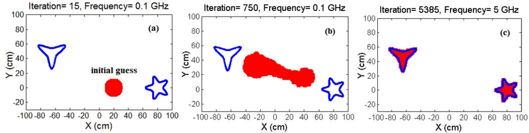
Fig. 1. Reconstruction of two cylinders, (a)initial guess, (b) after 750 iterations, (c) final result
