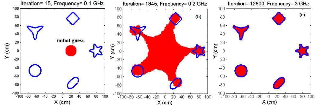
Fig. 4. Reconstruction of four cylinders, (a)initial guess, (b) after 1845 iterations, (c) final result
