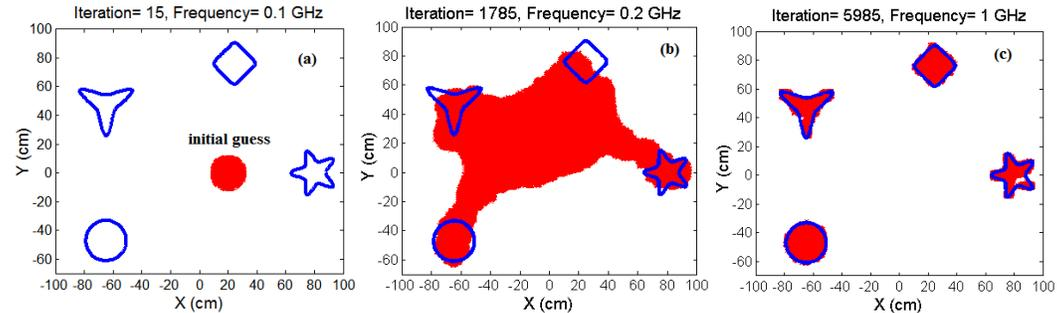
Fig. 3. Reconstruction of four cylinders, (a)initial guess, (b) after 1785 iterations, (c) final result
