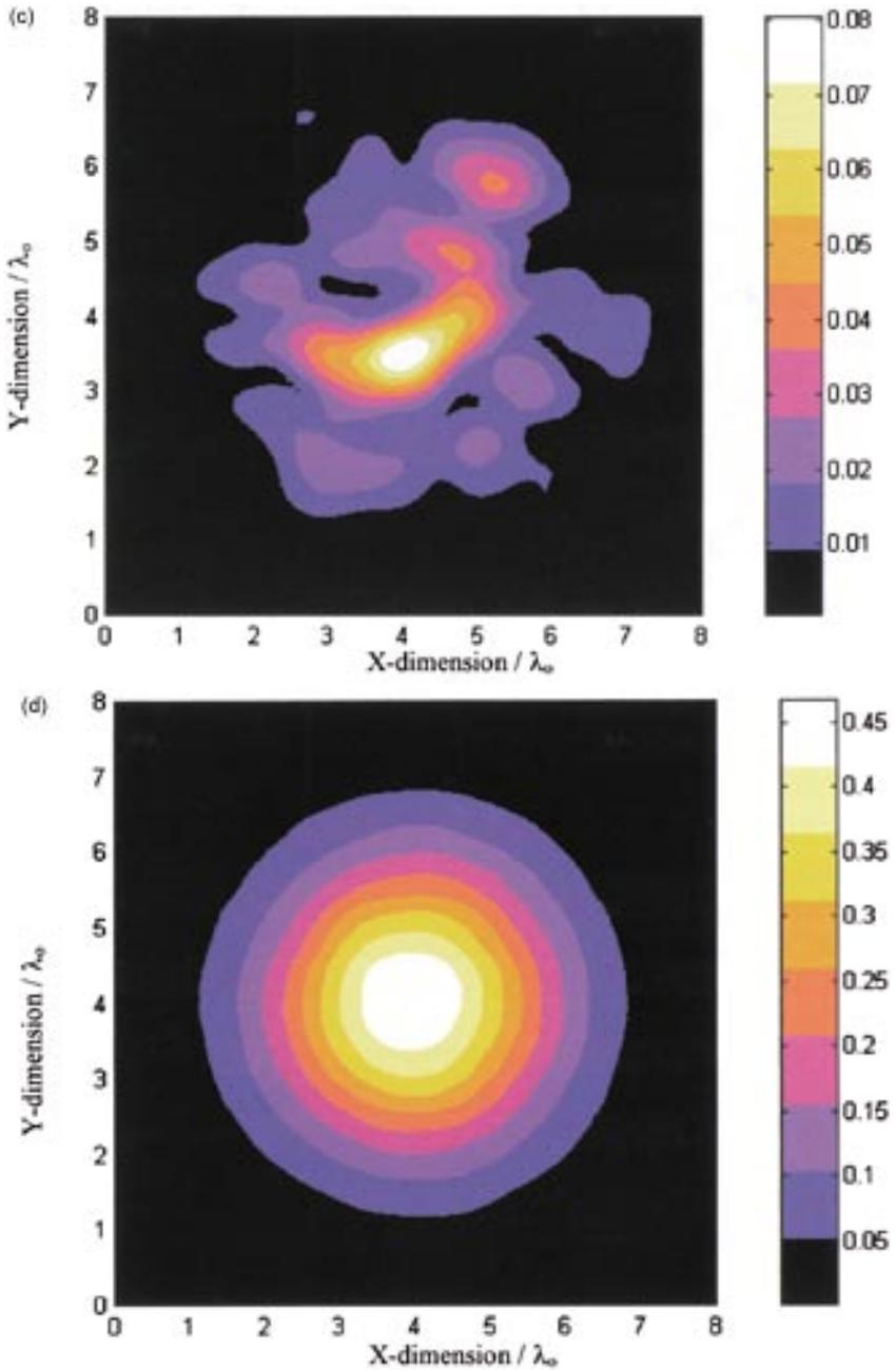
**Figure 3** (continued). c) Near field scattered at  $z = 1\lambda_0$  above the mean ground of Bosnian soil rough surface of root mean square height  $\sigma = 0.17\lambda_0$  and correlation length  $l_c = 1\lambda_0$ , and incident angle  $\theta' = 0$ . d) Near field transmitted at  $z = -1\lambda_0$  below the mean ground of Bosnian soil rough surface of root mean square height  $\sigma = 0.1\lambda_0$  and correlation length  $l_c = 1\lambda_0$ , and incident angle  $\theta' = 0$ .
