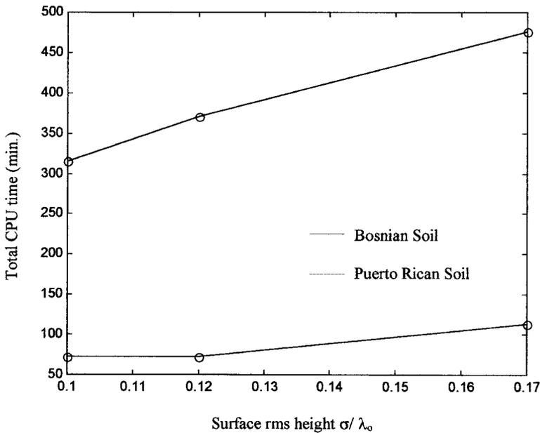
Figure 5. Total CPU time vs. the rms height of the rough surface.
