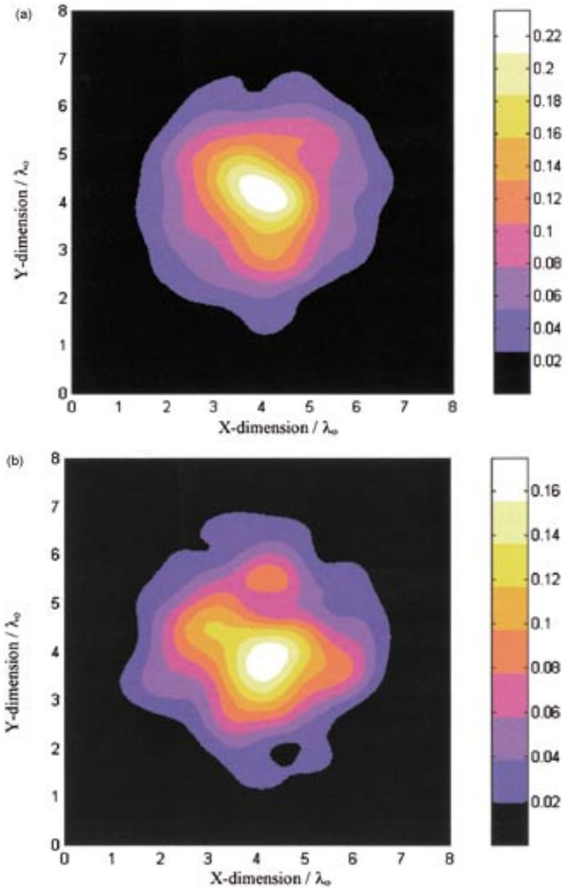
**Figure 4.** a) Near field scattered at  $z = 1\lambda_0$  above the mean ground of Puerto Rican soil rough surface of root mean square height  $\sigma = 0.1\lambda_0$  and correlation length  $l_c = 1\lambda_0$ , and incident angle  $\theta' = 0$ . b) Near field scattered at  $z = 1\lambda_0$  above the mean ground of Puerto Rican soil rough surface of root mean square height  $\sigma = 0.12\lambda_0$  and correlation length  $l_c = 1\lambda_0$ , and incident angle  $\theta' = 0$ .
