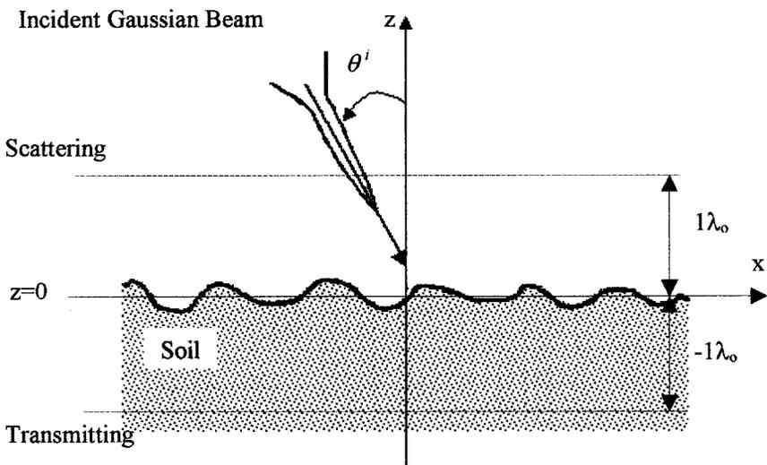
Figure 1. Cross section of rough soil ground with Gaussian beam incident at  $\theta'$ .
