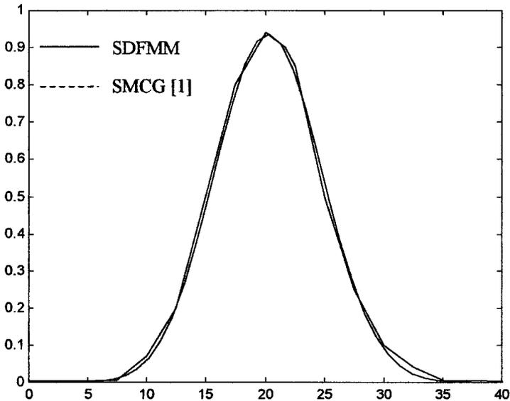
**Figure 2.** Normalized RCS for a rough surface of root mean square height  $\sigma = 0.02\lambda_0$  and correlation length  $l_c = 0.5\lambda_0$ , at incident angle  $\theta^i = 20^\circ$ . HH polarization.
