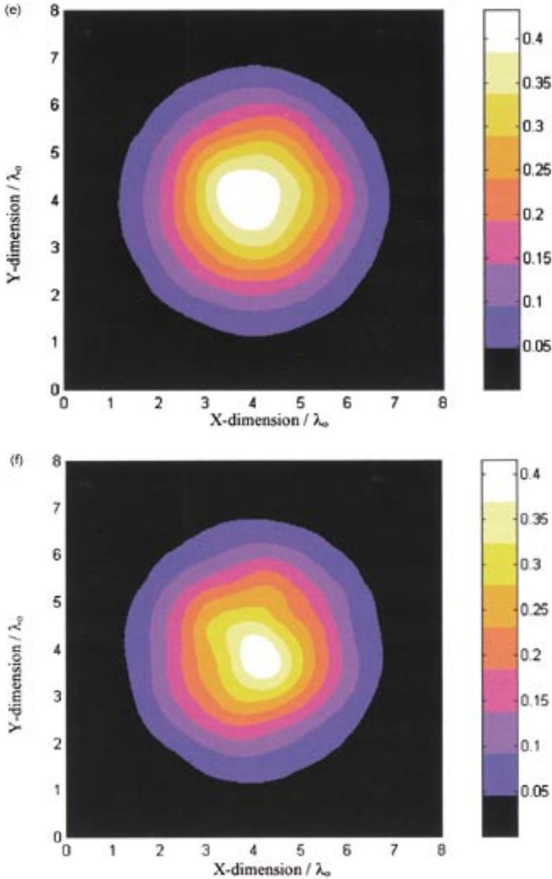
**Figure 3** (continued). e) Near field transmitted at  $z = -1\lambda_0$  below the mean ground of Bosnian soil rough surface of root mean square height  $\sigma = 0.12\lambda_0$  and correlation length  $l_c = 1\lambda_0$ , and incident angle  $\theta^i = 0$ . f) Near field transmitted at  $z = -1\lambda_0$  below the mean ground of Bosnian soil rough surface of root mean square height  $\sigma = 0.17\lambda_0$  and correlation length  $l_c = 1\lambda_0$ , and incident angle  $\theta^i = 0$ .
