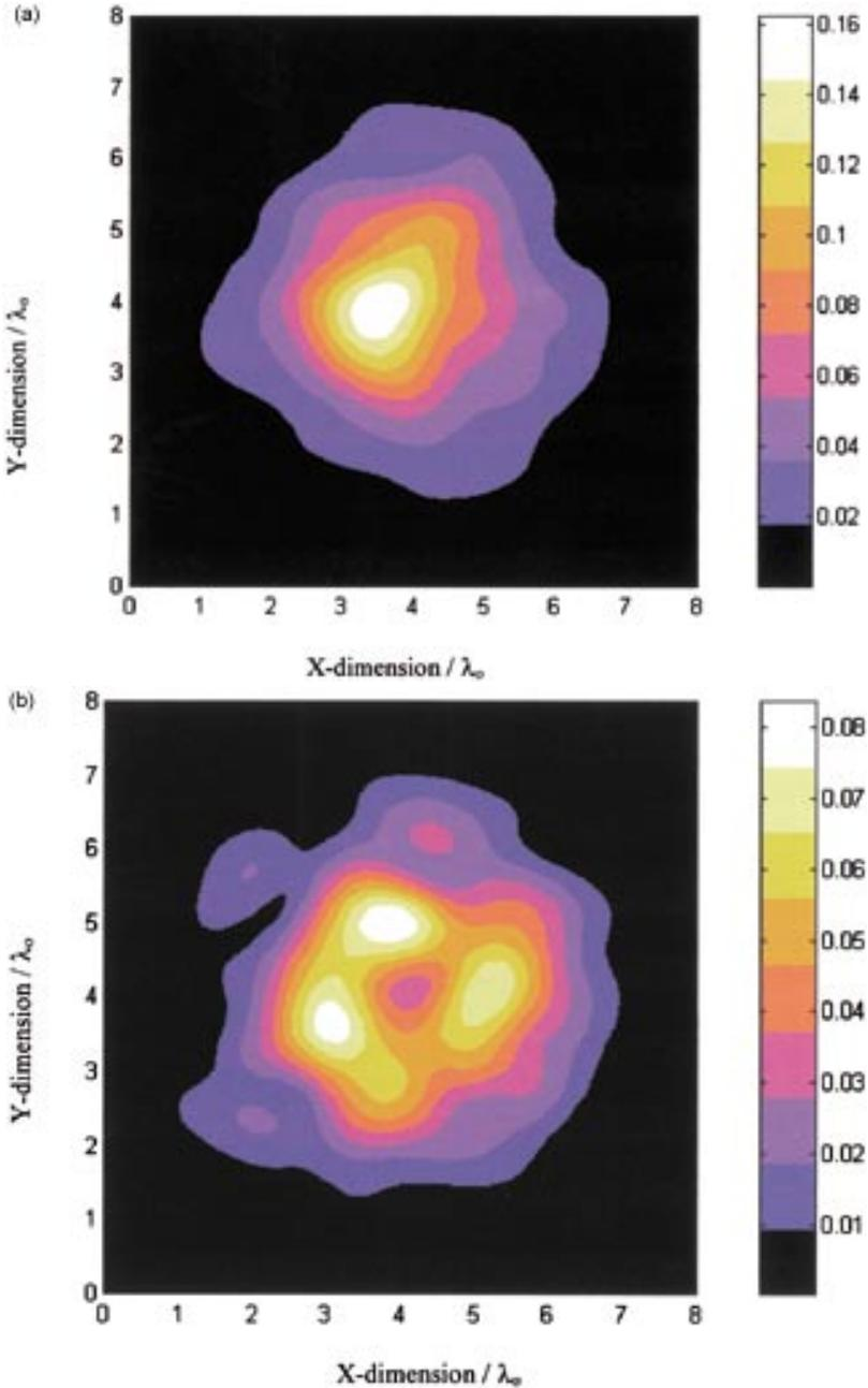
**Figure 3.** a) Near field scattered at  $z = 1\lambda_0$  above the mean ground of Bosnian soil rough surface of root mean square height  $\sigma = 0.1\lambda_0$  and correlation length  $l_c = 1\lambda_0$ , and incident angle  $\theta^i = 0^\circ$ . b) Near field scattered at  $z = 1\lambda_0$  above the mean ground of Bosnian soil rough surface of root mean square height  $\sigma = 0.12\lambda_0$  and correlation length  $l_c = 1\lambda_0$ , and incident angle  $\theta^i = 0^\circ$ .
