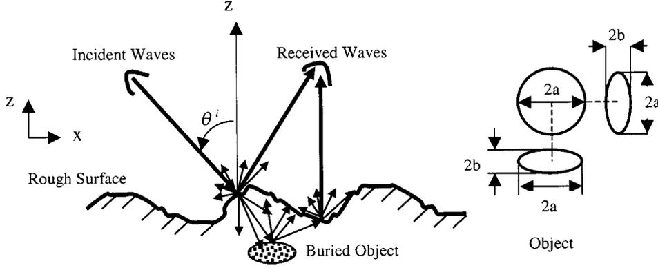
Fig. 1. Cross section of 3-D object buried under the rough surface ground. The object is modeled as oblate spheroid as:  $x = a \sin(\vartheta) \cos(\phi)$ ,  $y = a \sin(\vartheta) \sin(\phi)$ , and  $z = b \cos(\vartheta)$ .
