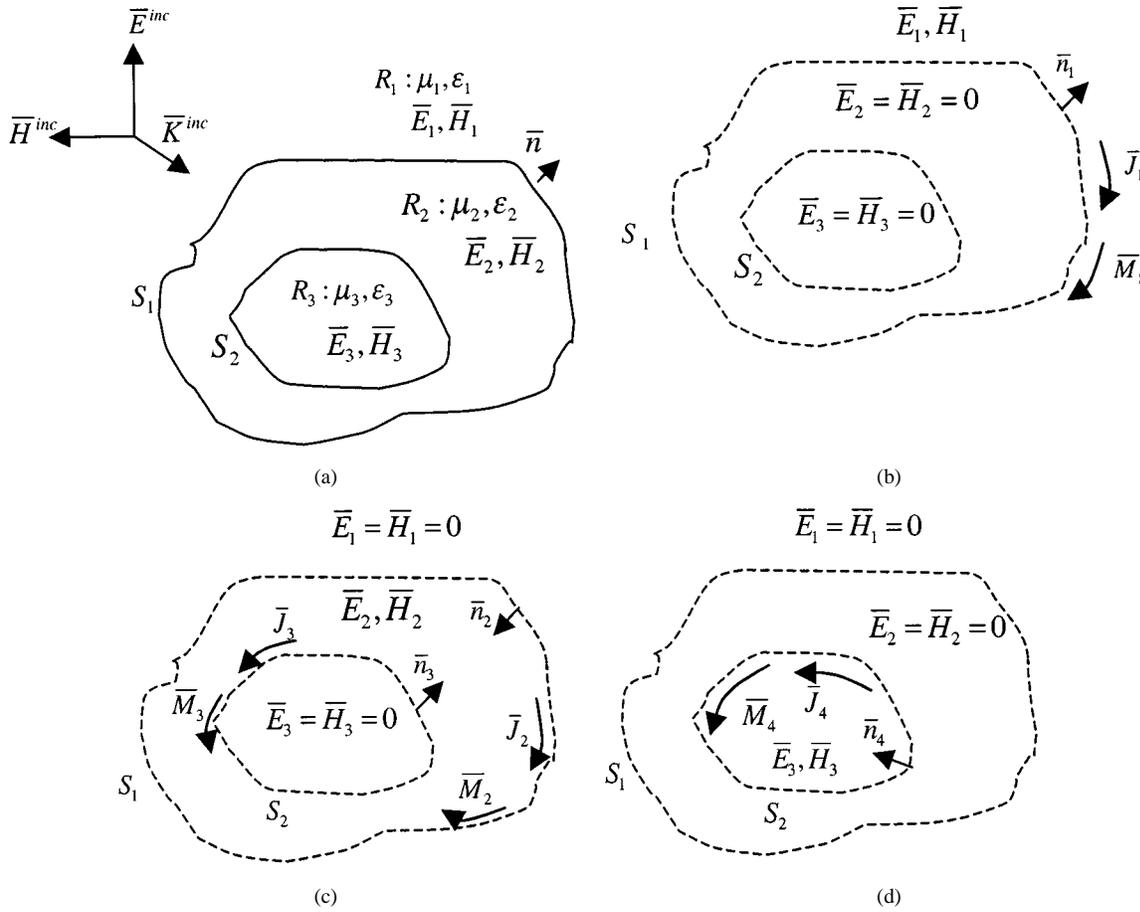
Fig. 2. (a) General penetrable 3-D scatterers  $R_2$  and  $R_3$ . (b) Equivalent problem exterior to  $S_1$ . (c) Equivalent problem interior to  $S_1$  and exterior to  $S_2$ . (d) Equivalent problem interior to  $S_2$ .
