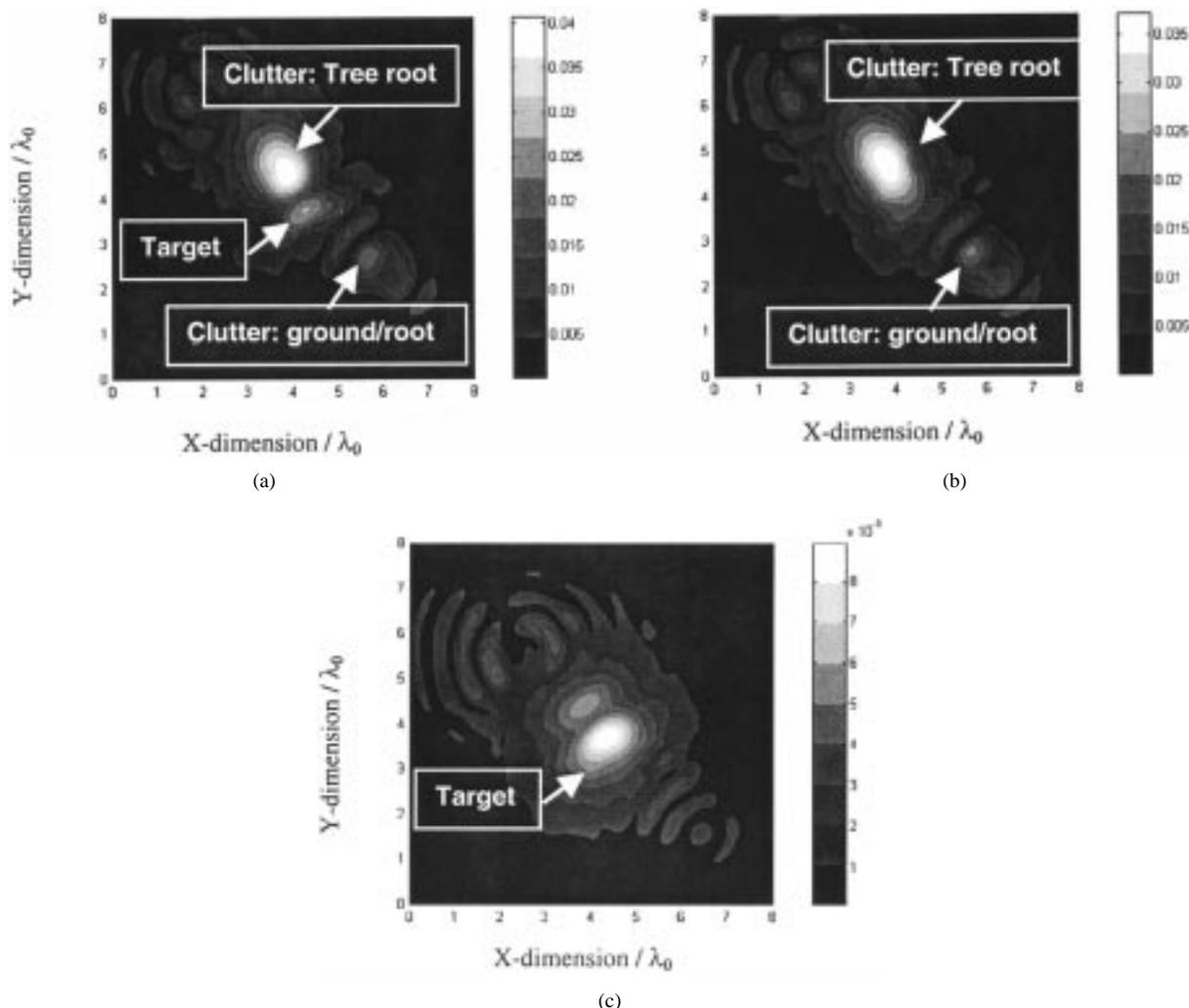
Fig. 5. Average scattered electric field upon removing the scattering from the rough ground for: (a) both the mine-like target and tree root, (b) just the tree root, and (c) just the mine-like target. Data are from Fig. 3(c) (H-polarization).
