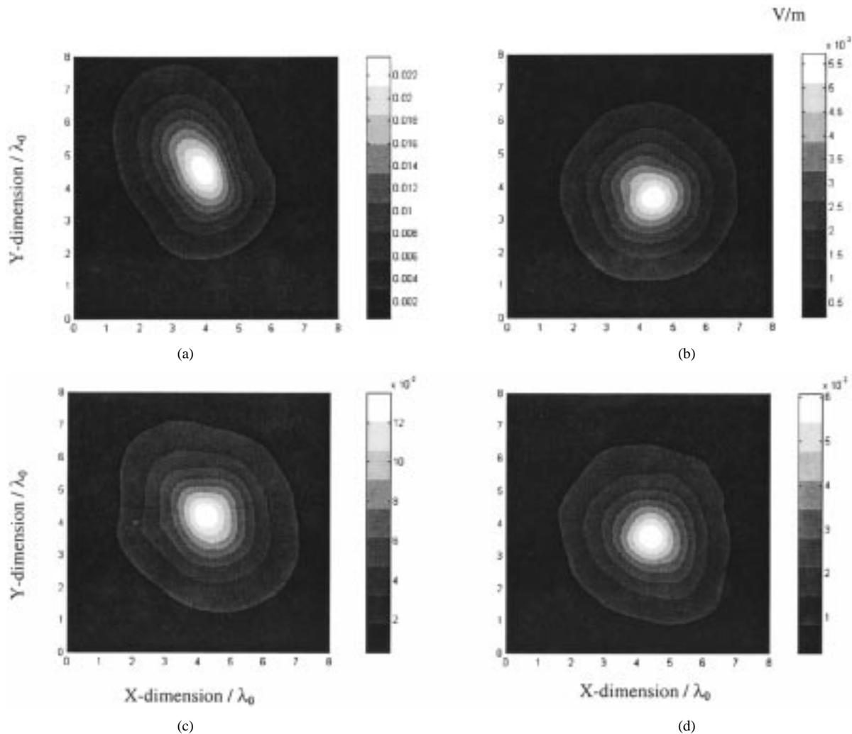
Fig. 8. Standard deviation of the scattered electric fields for (a) just the tree root, (b) just the AP-mine-like target, for the H-polarization, (c) just the tree root, and (d) just the AP-mine-like target, for the V-polarization. Data are from Fig. 3(c).
