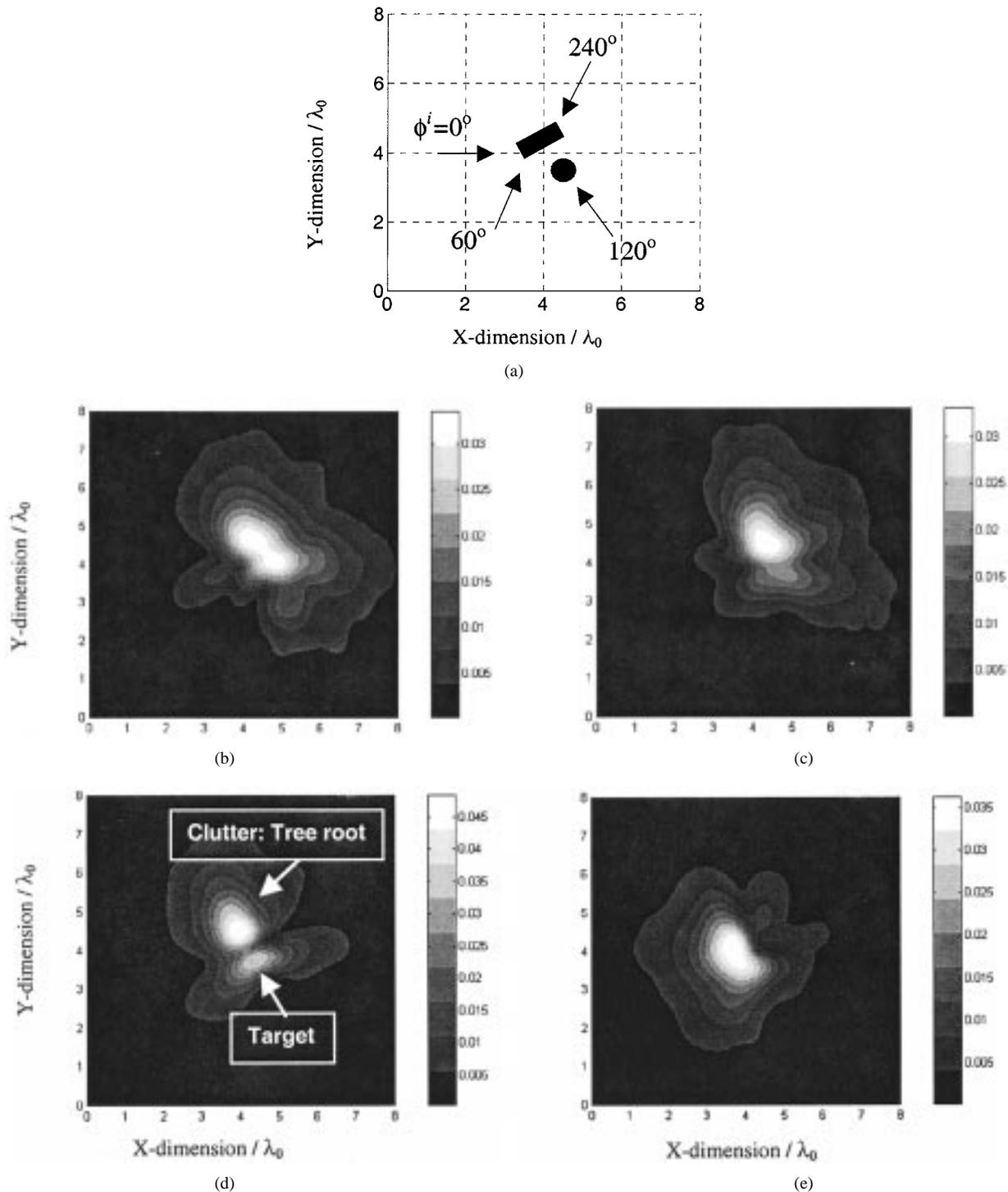
Fig. 3. (a) Top view of the target (oblate spheroid) and the tree root (horizontal cylinder), (b-e) The scattered electric field at multiple views for both the buried mine-like target and the tree root upon removing the scattering from ground when: (b)  $\phi^i = 0^\circ$ , (c)  $\phi^i = 60^\circ$ , (d)  $\phi^i = 120^\circ$ , and (e)  $\phi^i = 240^\circ$ . All results are for  $\sigma = 0.1\lambda_0$ ,  $l_c = 0.5\lambda_0$ ,  $\theta^i = 30^\circ$  and H-polarization.
