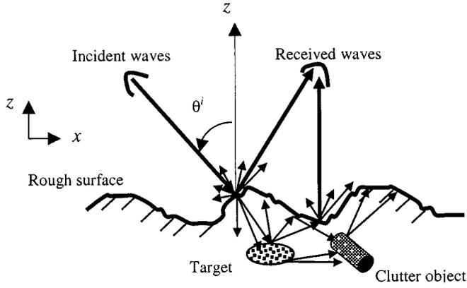
Fig. 1. Cross section of a target buried near a clutter object beneath the rough ground surface.
