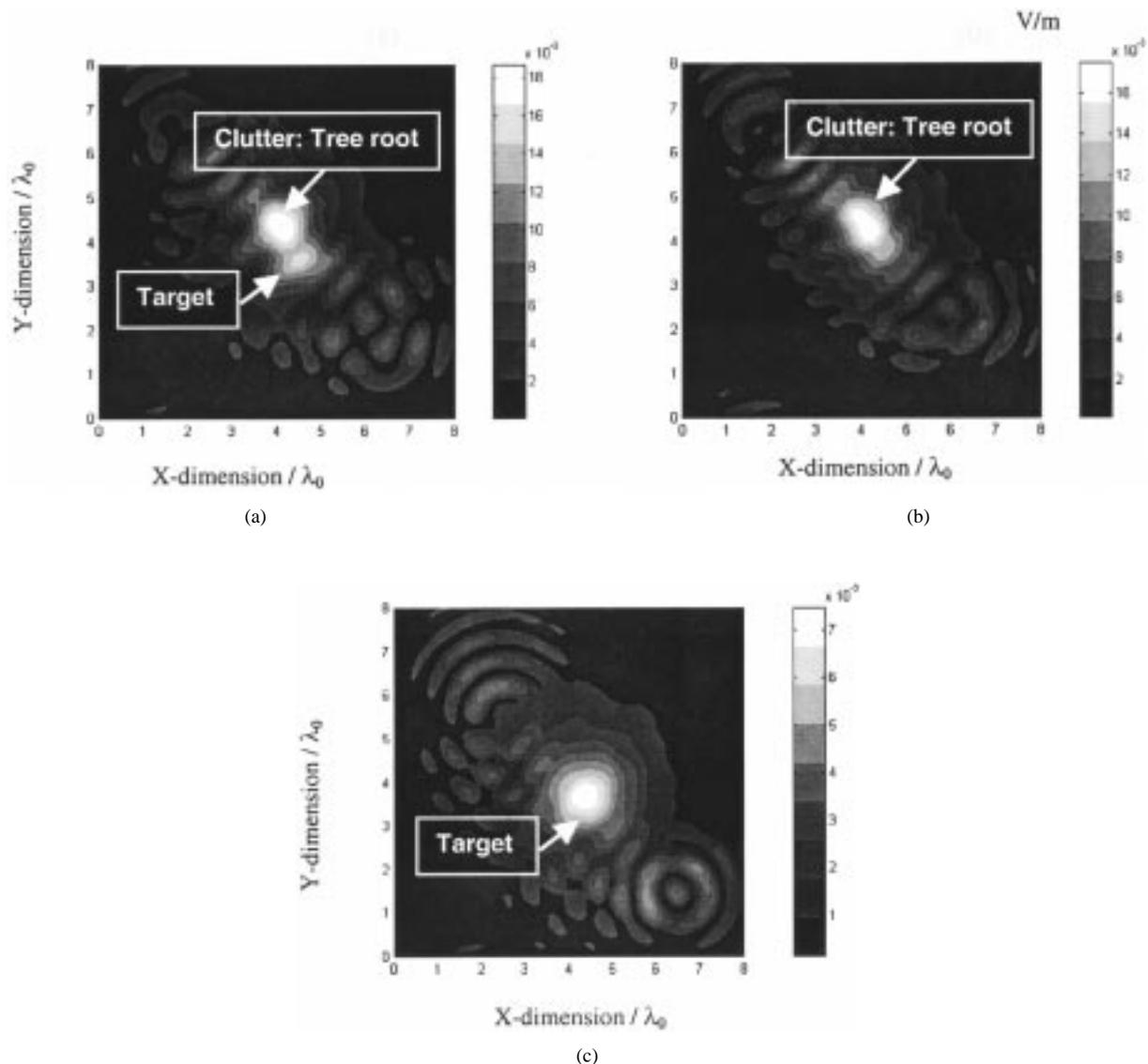
Fig. 7. Average scattered electric field upon removing the scattering from the rough ground for: (a) both the mine-like target and tree root, (b) just the tree root, and (c) just the mine-like target. Data are from Fig. 3(c) but for V-polarization.
