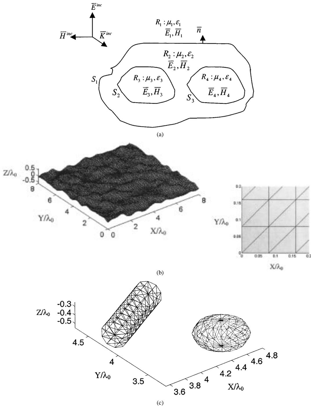
Fig. 2. (a) Two scatterers,  $R_3$  and  $R_4$ , immersed in region  $R_2$  immersed in region  $R_1$  and (b) triangular mesh for the rough ground (upper figure), for the oblate spheroid and the horizontal cylinder (lower figure).
