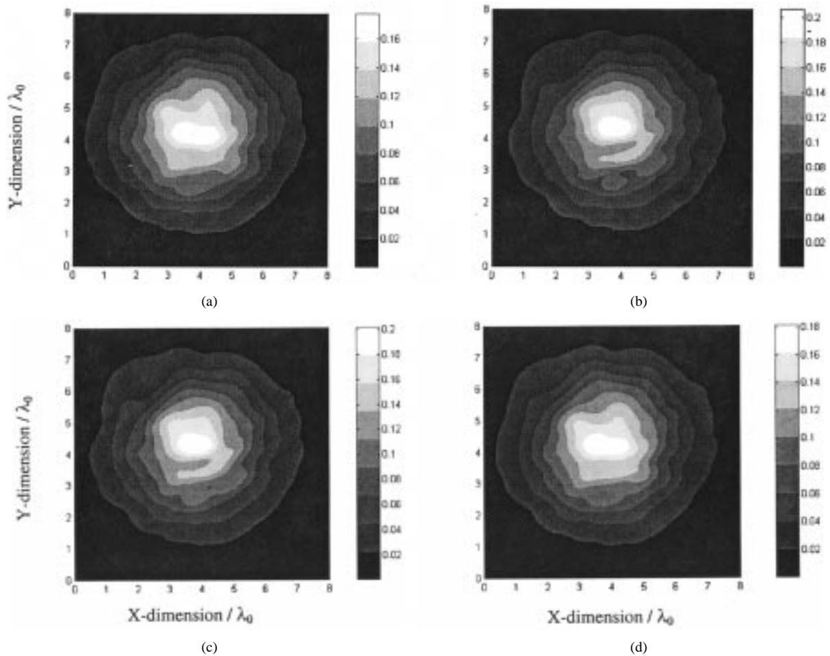
Fig. 4. Average scattered electric field at  $z = 0.5\lambda_0$  from: (a) the ground with no buried objects, (b) the ground with both the buried mine-like target and tree root, (c) the ground with only the buried tree root (no mine), and (d) the ground with only the buried mine-like target (no tree root). Data are from Fig. 3(c) (H-polarization).
