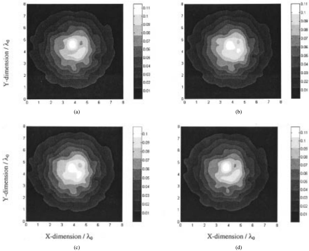
Fig. 6. Average scattered electric field at  $z = 0.5\lambda_0$  from: (a) the ground with no buried objects, (b) the ground with both buried the mine-like target and tree root, (c) the ground with only the buried tree root (no mine), and (d) the ground with only the buried mine-like target (no tree root). Data are from Fig. 3(c) for V-polarization.
