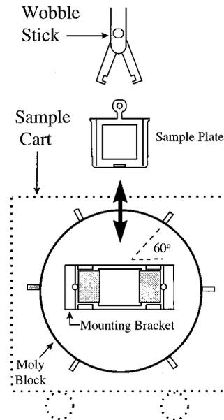
FIG. 2. A schematic explosion-style diagram showing the wobble stick, sample plate, and MBE moly block with a mounting bracket attached. The wobble stick moves along the face of the MBE moly block to position the sample on or off the mounting bracket.
