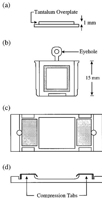
FIG. 1. Schematic diagrams showing the modified sample plate and mounting bracket. (a) Side view of modified sample plate showing 1 mm thick tantalum over plate. (b) Front view of modified sample plate. (c) Front view of standard mounting bracket used to hold the tantalum sample plate. (d) Side view of mounting bracket showing the compression clips which hold the STM sample plate.
