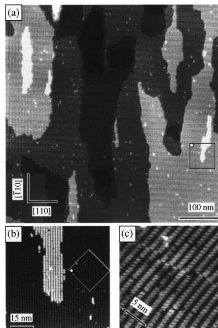
FIG. 4. Filled state STM images of a 1 μm thick GaAs film grown by MBE on a GaAs(001) substrate. (a) 1.5 μm × 1.5 μm area, with each gray level representing a change in height of 0.3 nm (a single GaAs layer). (b) 100 nm × 100 nm area zoom showing the 4-by periodicity of the (2×4) surface reconstruction. (c) 30 nm × 30 nm area zoom showing the 2-by periodicity of the surface reconstruction.
