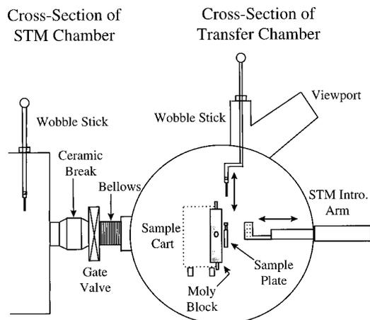
FIG. 3. Schematic diagram showing a cross-sectional view down the axis of the transfer chamber. This view shows how the wobble stick lifts the sample plate off the MBE moly block and positions it on the magnetic drive. Once the sample plate is on the magnetic drive it is moved underneath a second wobble stick inside the STM chamber, which removes the plate and positions it on the standard manipulator. In addition, the electrical break, gate valve, and vibration isolation bellows are shown.
