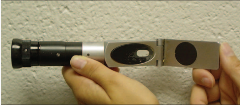
Figure 13. A handheld refractometer can be used in the vineyard as well as in the laboratory to determine sugar content of fruit and juice.
