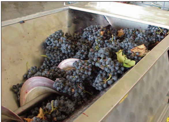
Figure 3. Destemming/crushing equipment removes the grapes from their stems and crushes the fruit to release the juice.
