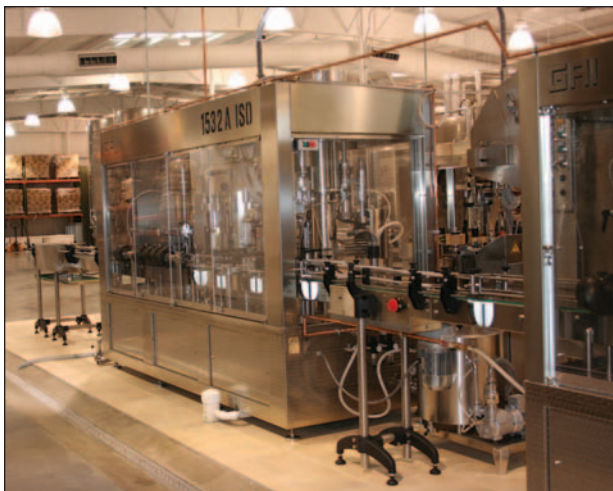
Figure 8. Fully automated bottling lines fill and cork the bottles before moving them directly into labeling machines. (Photo courtesy of Prospero Equipment Corp.)
