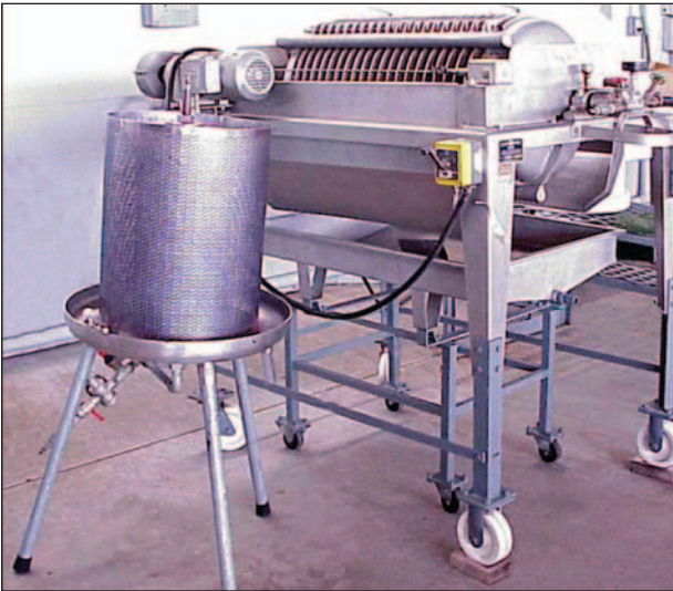
Figure 6. Horizontal and vertical presses are available in sizes ranging from the small capacity models shown here to large models capable of handling 20 tons of grapes at a time.
