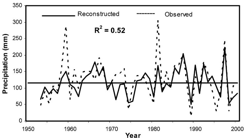
**Fig. 2** Time series comparison of observed and reconstructed winter-spring (January–June) precipitation for the period 1953–2000. This period was divided in half for two separate sets of calibration and validation, 1976–2000 and 1953–1975, before calibrating on the full 48 years period
