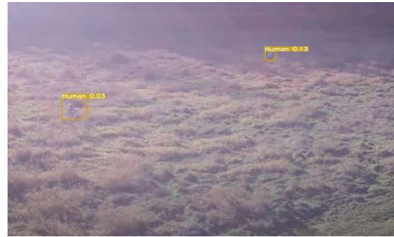
(b) Visual Lens Glare: From left to right the detections are 3% and 13% confident
