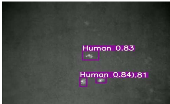
(a) Night Thermal with detections from right to left at 84%, 83%, and 81% confident.
