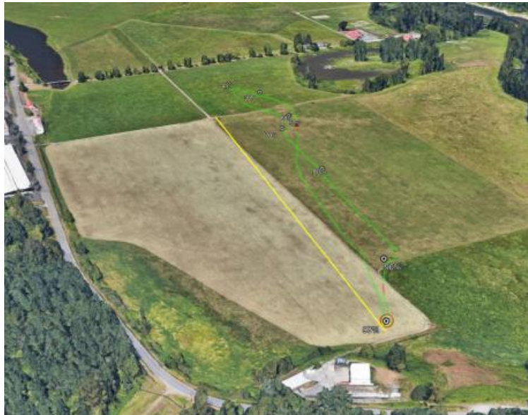
Fig. 19 The green line is the flight path of the sUAS and the yellow line is 500 m
