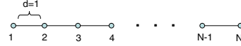
Fig. 5. Simple linear topology used to study the effect of model parameters on the correlation in data.
