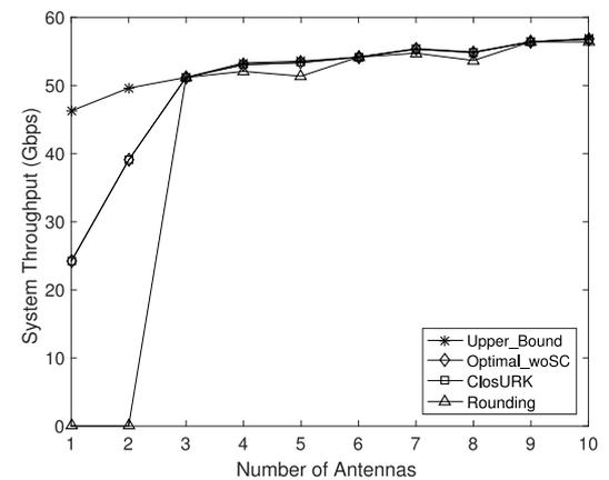
Fig. 5. System throughput of ClosURK v.s. number of antennas.
