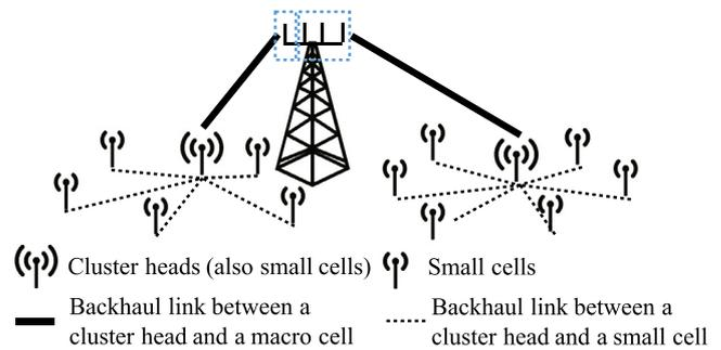
Fig. 1. Hybrid architecture.
