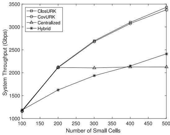
Fig. 13. System throughput of different architectures v.s. number of small cells.
