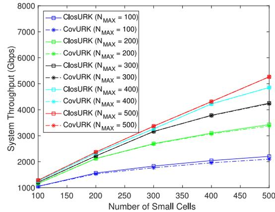
Fig. 12. System throughput of ClosURK and CovURK v.s. number of small cells.
