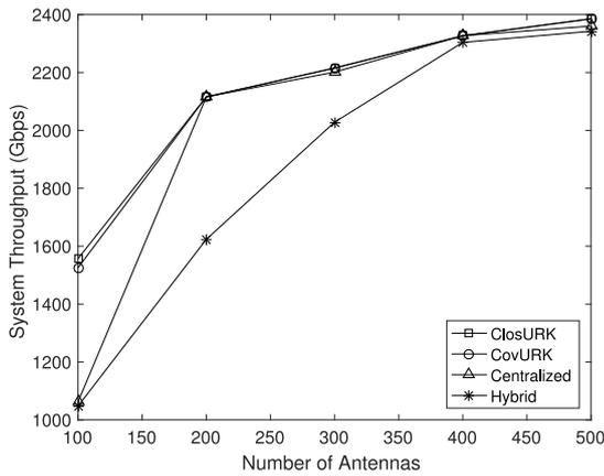
Fig. 14. System throughput of different architectures v.s. number of antennas.
