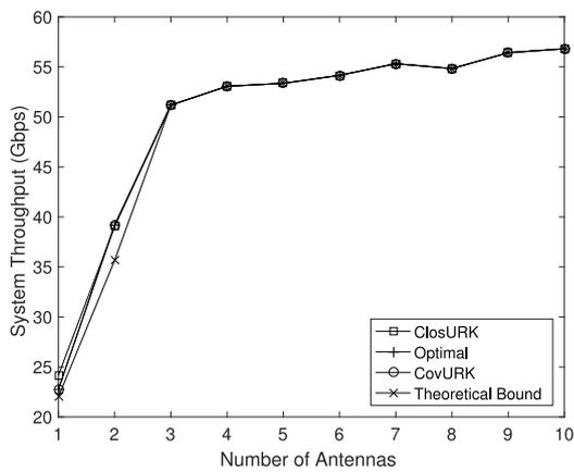
Fig. 7. System throughput of CovURK v.s. number of antennas.
