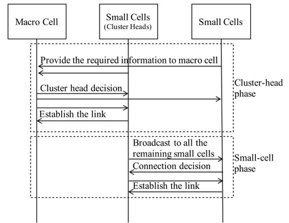
Fig. 15. Signaling flow for mmHAUL.
