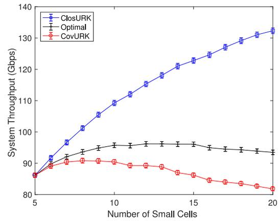
Fig. 11. System throughput with 95% confidence intervals v.s. number of small cells.
