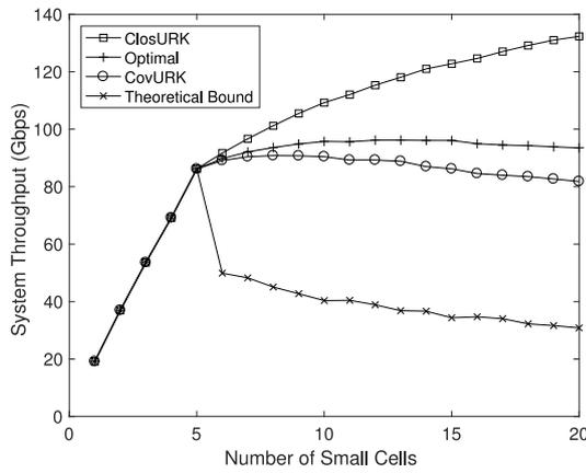
Fig. 6. System throughput of CovURK v.s. number of small cells. (Note that ClosURK does not satisfy the coverage constraints and this is why it is above the Optimal.).
