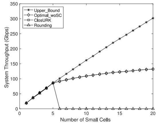
Fig. 4. System throughput of ClosURK v.s. number of small cells.
