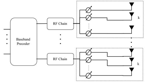
Fig. 16. Partially-Connected Hybrid Beamforming Architecture.
