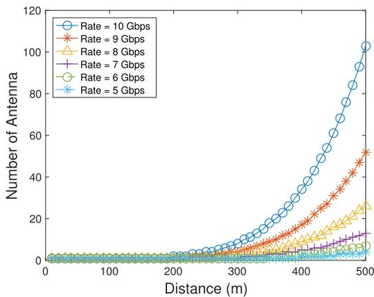
Fig. 2. Number of Required Antennas with Different Rate Requirement.
