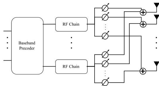
Fig. 3. Fully-Connected Hybrid Beamforming Architecture [37].
