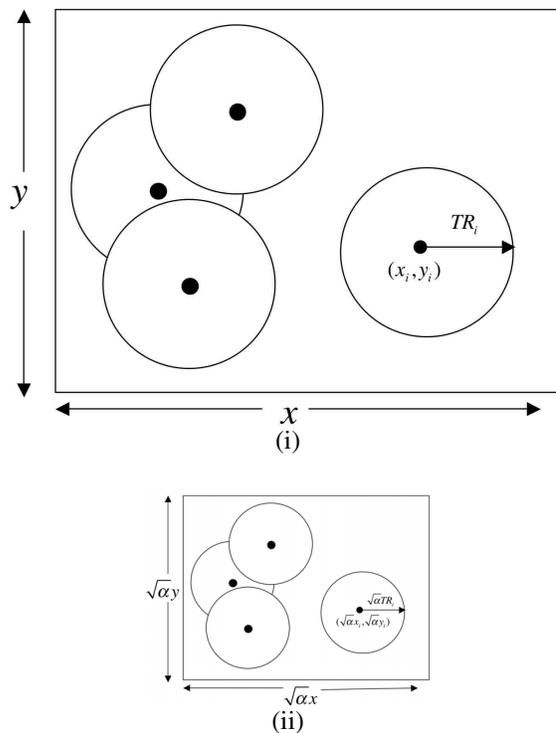
Fig. 1. (i) Original system (area size =  $A$  square units), and (ii) scaled-in-space system (area size =  $\alpha A$  square units). (In this example  $\alpha = 0.25$ .)
