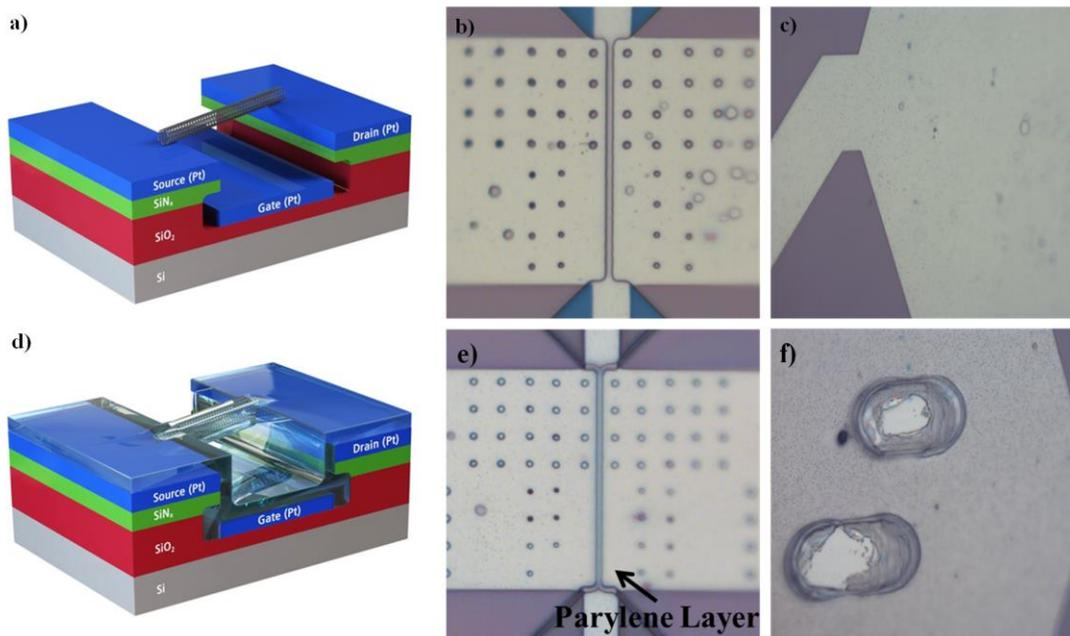
Fig. 1. Device schematic and optical microscope images of CNTFET. a) Device schematic, b) 500 nm channel, and c) contact pads before and d), e), and f) after parylene passivation with pockets made for probing. The parylene layer can clearly be seen in e) and f) and covers the entire device.
