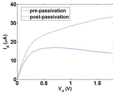
Fig. 5. Drain voltage sweep ( $V_g = -5$  V) of a metallic CNTFET before and after passivation showing the elimination of negative differential conductance (NDC) and higher currents.
