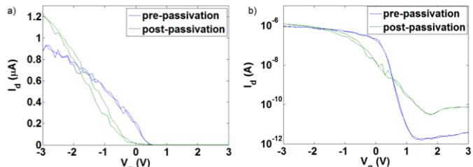
Fig. 2.  $I-V_g$  characteristic plot ( $V_d = 0.1V$ ) of the same CNTFET before and after parylene deposition (linear (a) and log (b)). Note negligible hysteresis along with the clear changes in threshold voltage, On/Off ratio, Off current, and subthreshold swing.
