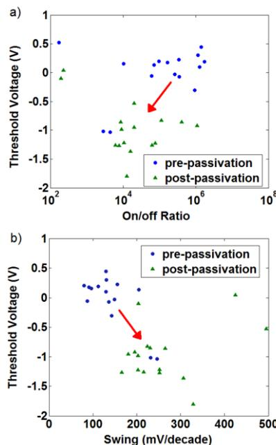
Fig. 4. Scatter plot of a) On/Off ratio versus threshold voltage and b) subthreshold swing versus threshold voltage both pre- and post-parylene passivation, showing a shift to higher swing, lower threshold voltages, and lower On/Off ratio.
