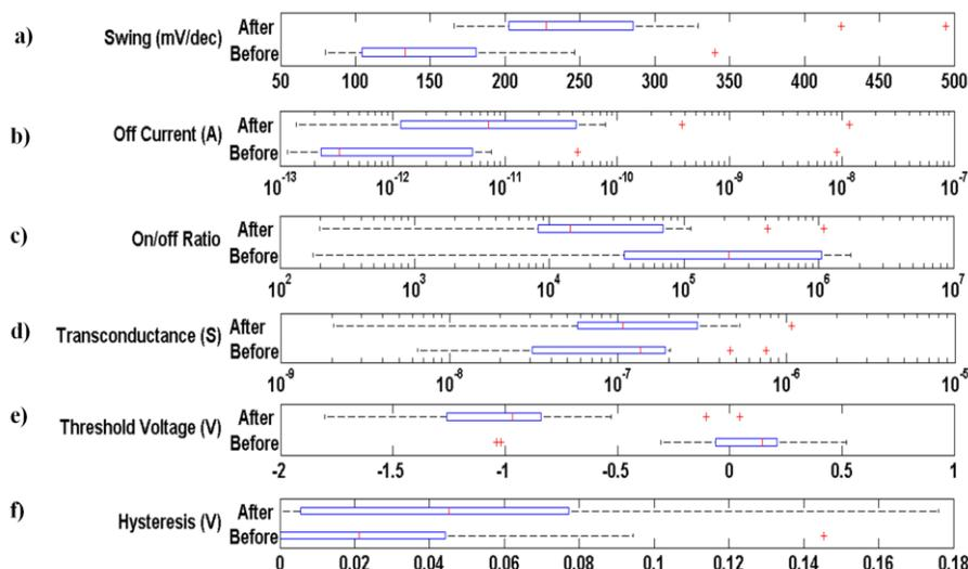
Fig. 3. Box plots of changes in electrical characteristics before and after passivation for 16 devices. a) swing, b) Off current, c) On/Off ratio, d) transconductance, e) threshold voltage and f) hysteresis width. Left and right box edge mark first and third quartiles. Middle red line marks the median. Outliers are marked as red crosses.
