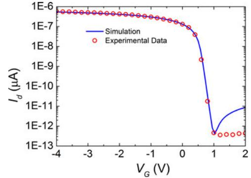
Fig. 2. Low voltage electrical transport data. Drain current versus gate voltage for a semiconducting CNT. Experimental data (red circles) and theoretical transport model (blue line) agree nicely for  $V_G < 1$  V.
