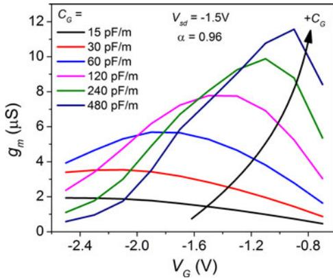
Fig. 7. Transconductance  $g_m$  versus gate voltage for several different gate capacitance values at a  $V_{sd} = -1.5$  V and  $\alpha = 96\%$ .
