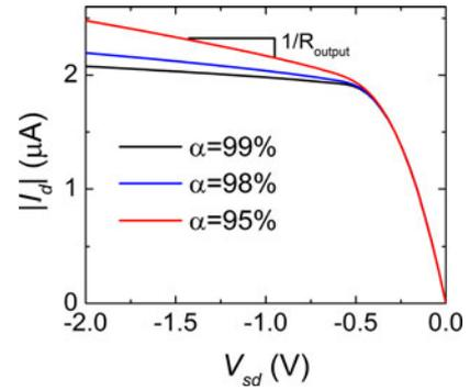
Fig. 5. Channel length modulation in a CNT FET. Drain current versus source-drain voltage at gate efficiencies  $\alpha$  of 99%, 98%, and 95%, showing decreased output resistance for lower gate coupling efficiencies caused by channel length modulation.
