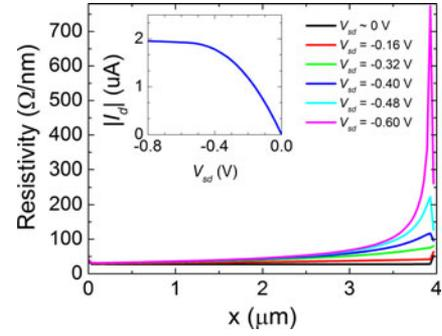
Fig. 4. Pinchoff in a CNT FET. Resistivity versus spatial position along the length of a CNT FET during development of the pinchoff condition. Inset shows drain current versus source-drain voltage for this calculation.
