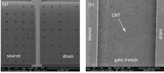
Fig. 1. CNT device geometry. (a) SEM images of CNT device layout and (b) close-up image of a single CNT crossing the trench.
