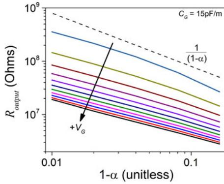
Fig. 6. Output resistance as a function of  $1-\alpha$  for different gate voltages ( $V_G = -2.6$  to  $-0.6$  V).  $R_{\text{output}}$  has a power law dependence on  $1-\alpha$ , with  $R_{\text{output}}$  increasing as  $\alpha \rightarrow 1$ .
