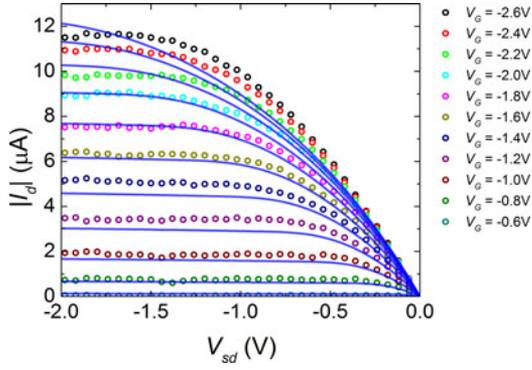
Fig. 3. High voltage electrical transport data. Experimental (open circles) and theoretical (blue lines) drain current plotted versus source-drain voltage for various gate voltages. The experimental data is from [25] (reprinted with permission).
