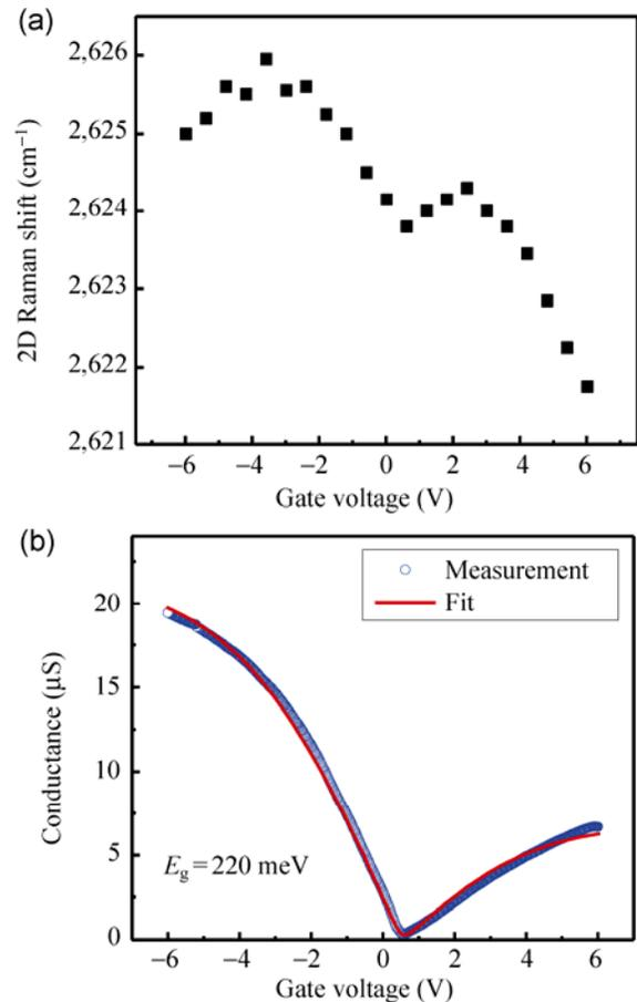
**Figure 2** (a) Gate voltage dependence of the 2D band Raman shift and (b) conductance–gate voltage curve for a suspended metallic CNT measured at room temperature.
