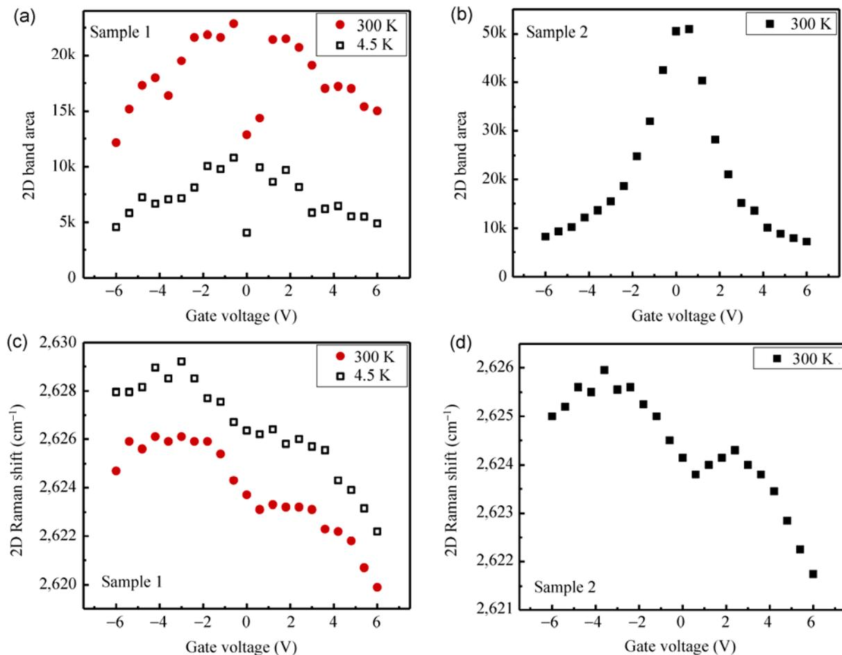
**Figure 5** (a), (b) 2D band Raman integrated area intensities and (c), (d) Raman shifts for two different quasi-metallic devices (Sample 1 and Sample 2).
