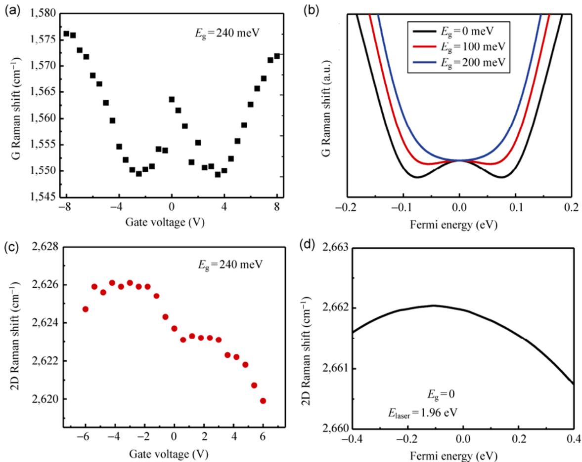
**Figure 4** Experimentally measured (a) G and (c) 2D Raman modes taken from the same nanotube at room temperature. Non-adiabatic calculations of the gate dependence of the (b) G and (d) 2D bands.
