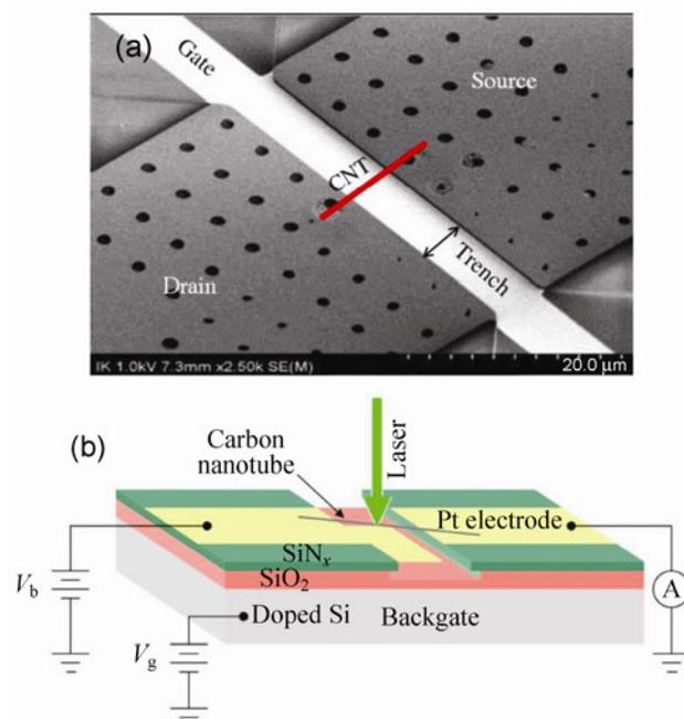
**Figure 1** (a) Scanning electron microscope image and (b) schematic diagram of suspended carbon nanotube field effect transistor device.
