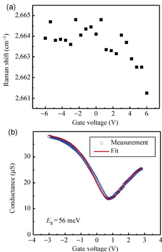
**Figure 3** (a) Gate voltage dependence of the 2D band Raman shift and (b) conductance-gate voltage curve for another suspended quasi-metallic CNT measured at room temperature.
