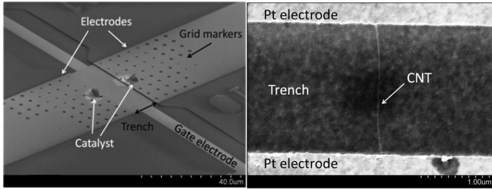
**Figure 1.** SEM images of a suspended CNT sample device. The right panel shows a high resolution SEM image of an individual carbon nanotube.
