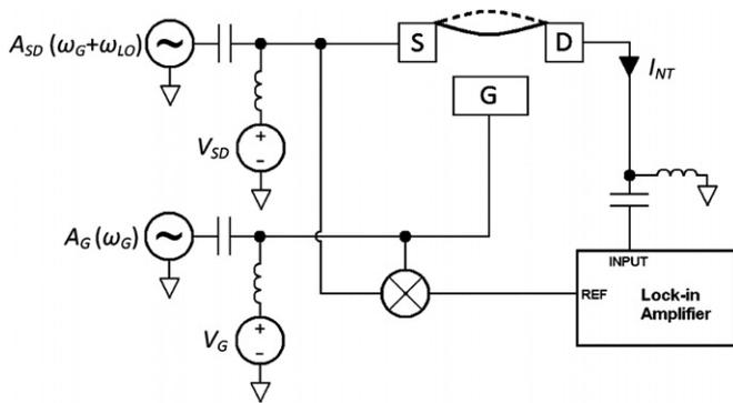
**Figure 2.** Circuit diagram of the electromechanical resonator setup.
