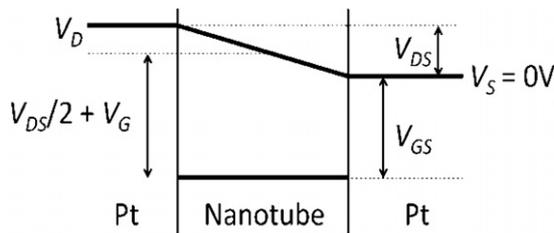
**Figure 5.** Effective gating of the CNT due to asymmetric source-drain bias voltage.
