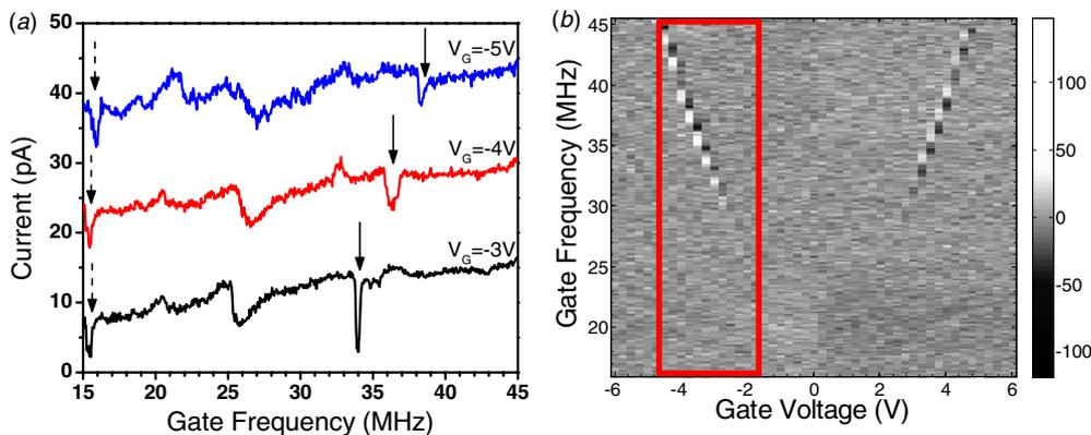
**Figure 3.** (a) Electric current plotted as a function of gate frequency. The solid arrows show the resonance due to the nanotube and dashed arrows point to resonances due to passive circuitry elements. (b) Electric current plotted as a function of the gate frequency ( $f_G$ ) and dc gate voltage. The red box corresponds to the experimental regime shown in figure 4(b).
