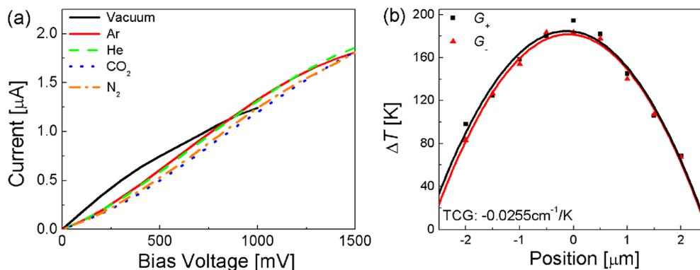
FIG. 2. (Color online) (a) Current-voltage curves of a 5  $\mu\text{m}$  long suspended CNT measured in vacuum and different gas environments. (b)  $G_+$  and  $G_-$  band phonon temperature distributions measured along the suspended CNT in argon under an electrical power of 2.67  $\mu\text{W}$ . The average  $G_+$  and  $G_-$  band phonon temperatures are 127 K and 123 K, respectively, along the suspended nanotube.
