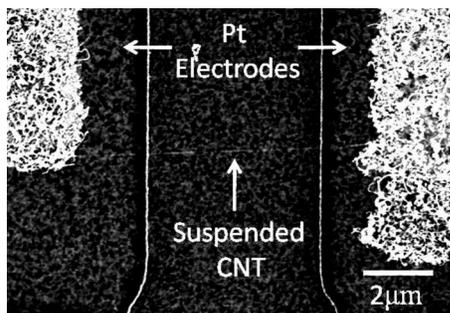
FIG. 1. SEM image of a 5  $\mu\text{m}$  long CNT suspended between two Pt electrodes.
