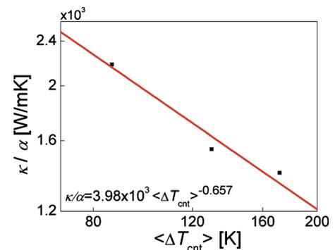
FIG. 5. (Color online) Measured  $k/\alpha$  as a function of the average CNT temperature,  $\langle \Delta T_{\text{cnt}} \rangle$ , extracted from  $G$  band downshifts measured during electrical heating.
