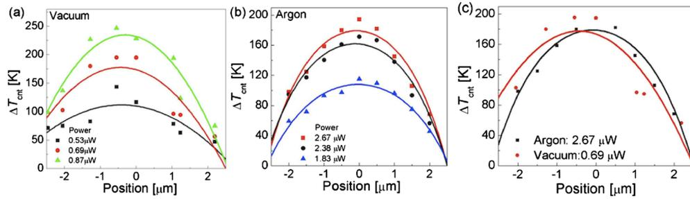
FIG. 3. (Color online) Temperature profiles along the CNT measured in Fig. 2 under various electrical heating powers (a) in vacuum and (b) in argon. (c) Comparison of heating powers required in argon and in vacuum to achieve approximately the same temperature in the nanotube.
