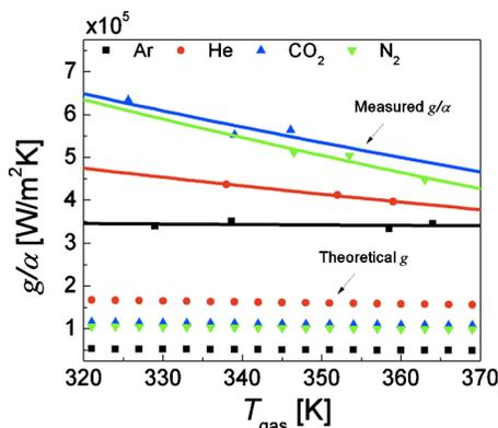
FIG. 6. (Color online) Measured  $g/\alpha$  as a function of the gas temperature  $T_{\text{gas}} \equiv (\Delta T_{\text{cnt}})/2 + 300$  K. Solid lines show  $T_{\text{gas}}^{-1/2}$  fitting to the measurement results (symbols). The symbols without the fitting lines are the theoretical  $g$  values from kinetic theory, proportional to  $T_{\text{gas}}^{-1/2}$ .
