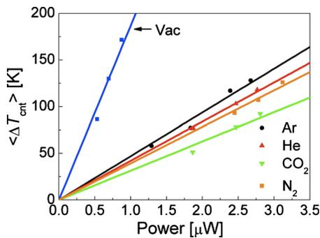
FIG. 4. (Color online) Average temperature of the CNT measured in different gases plotted with respect to power in different environments.
