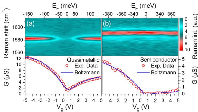
FIG. 3 (color online). The  $G$  band spectra and conductance ( $G$ ) for suspended (a) qm- and (b) sc-SWNTs, plotted versus  $V_g$  and  $E_F$ .  $G$  and  $E_F$  are fit using the Boltzmann-Landauer transport model.
