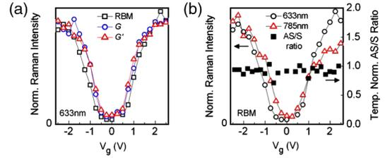
FIG. 2 (color online). (a) Normalized Raman intensities of the RBM,  $G_+$  (TO), and  $G'$  bands taken with a 633 nm laser. (b) RBM intensity taken with 633 and 785 nm lasers, together with the RBM AS/S intensity ratio (633 nm, normalized for  $T = 300 \text{ K}$ ) plotted versus  $V_g$ .
