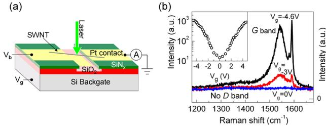
FIG. 1 (color online). (a) Device geometry and (b)  $G$  band Raman spectra at various gate voltages, with the inset showing the  $G_-$  band intensity as a function of  $V_g$  (sample 8B).
