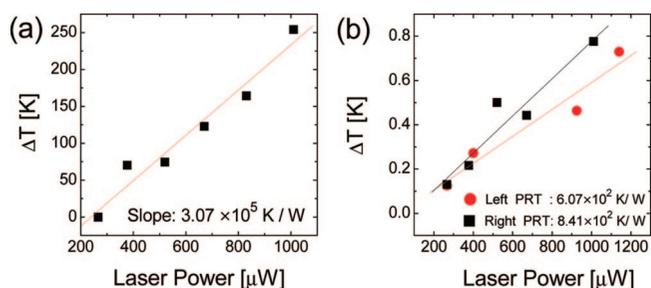
**Figure 4.** (a) Temperature in the center of the SWNT bundle shown in Figure 2 extracted from the G band downshifts plotted vs laser power. (b) Temperature of the left and right PRTs as a function of incident laser power.
