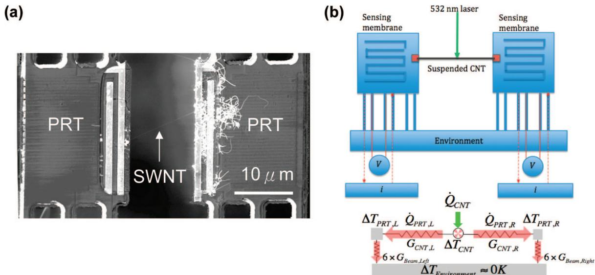
**Figure 1.** (a) Scanning electron microscopy image of microfabricated SiN<sub>x</sub> membranes with platinum resistance thermometers (PRTs) bridged by a SWNT bundle. (b) Schematic diagram of the experimental setup and thermal resistance circuit.
