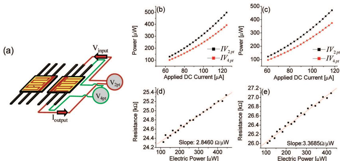
**Figure 3.** (a) Schematic diagram of the experimental setup for the PRT's electrical self-heating calibration. (b, c) Calibration data of the self-heating power plotted as a function of direct current for two-point and four-point measurements of the left and right PRTs. (d, e) Resistance of the left and right thermometers as a function of electric power, corrected for the effects of Joule heating in the leads.
