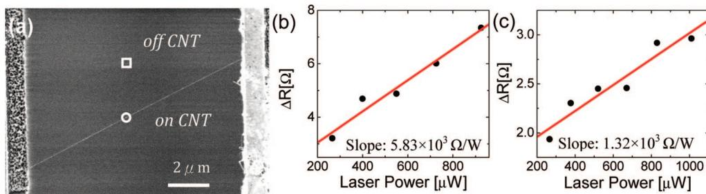
**Figure 2.** (a) Scanning electron microscopy image of a SWNT bundle suspended across an 11 μm trench. The circle and square represent the location of laser spot *on* and *off* the SWNT, respectively. (b, c) Resistance change with increasing laser power *on* and *off* the SWNT for the left and right thermometer, respectively.
