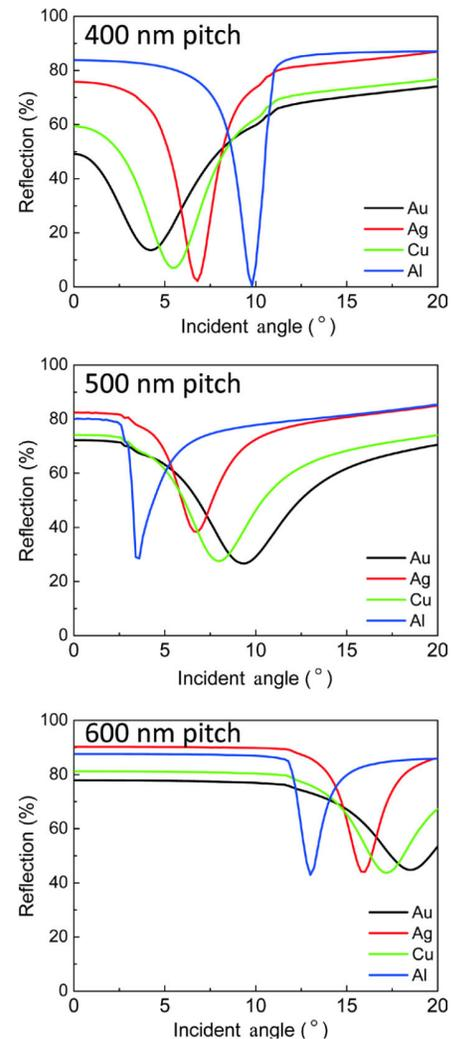
**Figure 4** FDTD simulations of reflection of 633 nm light for different metals and pitches at different incident angles.
