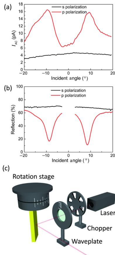
**Figure 2** Characterization of the plasmon resonant grating. (a) Photocurrent and (b) photoreflectance as a function incident angle for 633 nm light polarized parallel and perpendicular to the grating structure. (c) Schematic of the experimental measurement configuration.
