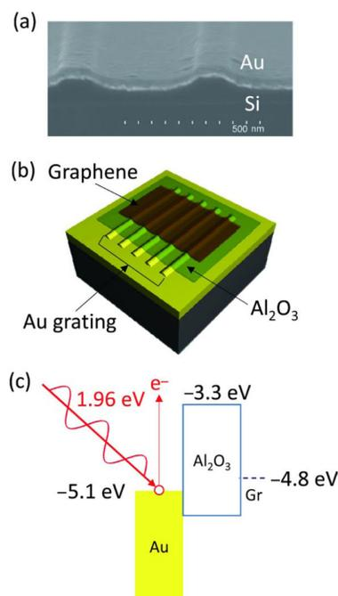
**Figure 1** Illustrations of plasmon resonant grating structure. (a) Cross-sectional SEM image and (b) schematic. (c) Energy band diagram with respect to vacuum illustrating the mechanism of hot electron injection.
