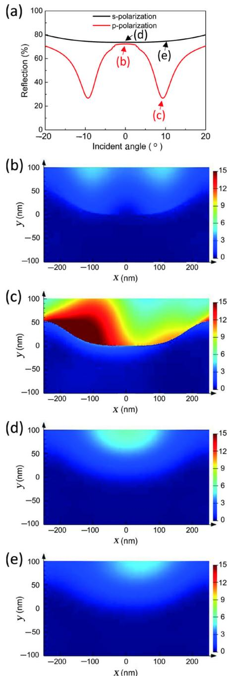
**Figure 3** FDTD simulation results for different incident conditions. (a) Simulated photorefectance as a function of incident angle for p- and s-polarized light. Simulated cross-sectional electric field intensity profiles ( $E^2$ ) for illumination at (b), (d) normal and ((c), (e)) 10° incidence.
