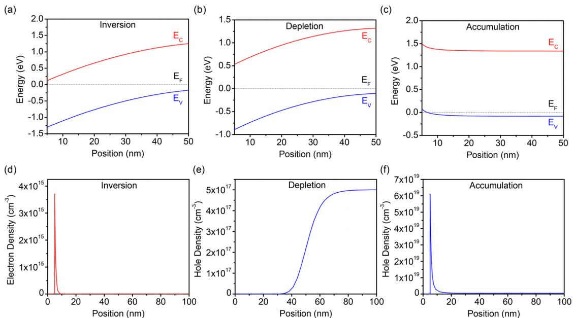
FIG. 3. Energy band diagrams and free carrier concentration of the semiconductor surface under (a) and (d) inversion, (b) and (e) depletion, and (c) and (f) accumulation conditions.
