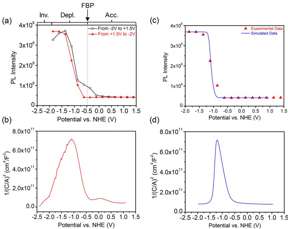
FIG. 2. (a) The photoluminescence intensity and (b) Mott-Schottky ( $1/C^2$  vs.  $V$ ) plot of a  $\text{TiO}_2$ -passivated GaAs photocathode measured as a function of the reference potential. [(c) and (d)] Simulated results for a GaAs photocathode over the same voltage range.
