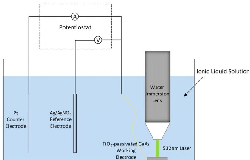
FIG. 1. Schematic diagram of the three-terminal photoelectrochemical cell. The water immersion lens is mounted on a microscope in the spectrometer for photoluminescence measurements.
