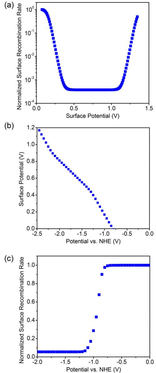
FIG. 4. (a) The normalized recombination rate of a GaAs semiconductor as a function of surface potential under illumination. (b) The surface potential plotted as a function of NHE extracted from the TCAD simulation. (c) The expected recombination rate as a function of applied bias under illumination.
