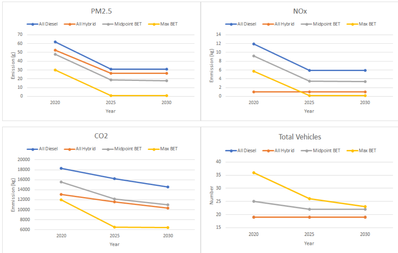
Figure 6: Emissions and total vehicles per day for four vehicle scenarios, each target year
