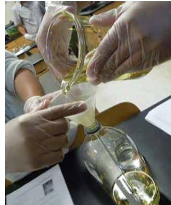
3. Using a beaker measure out 200 ml of methanol and pour into an empty mason jar. Use your gloves and goggles while pouring the methanol and cap the bottle containing the methanol tightly afterwards to avoid inhaling fumes.
