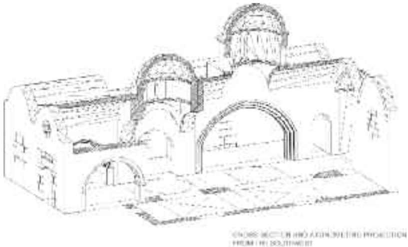
Fig. 8: Trapeza church, axonometric projection from the southwest showing 14 th century dome (left) and 16 th century dome (right) (projection by Joanna Ostrowska)
