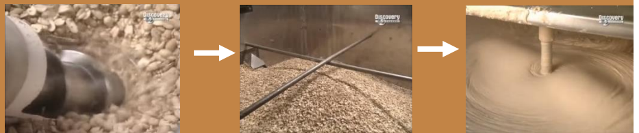
Figure 6- The peanuts are reduced to a medium grind first, then into a fine, smooth texture.
