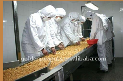
Figure 5- The peanuts are being inspected by the workers, who remove the defected nuts.
