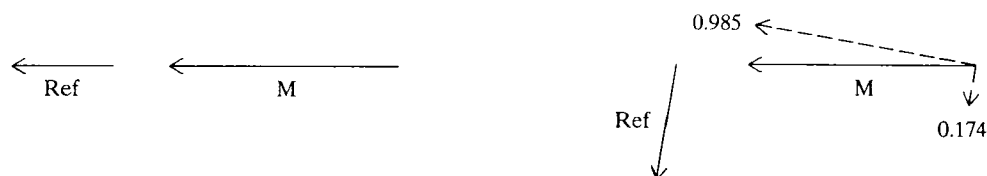
Figure 8. Vector diagrams for real and imaginary references phase-shifted by only 80^\circ , instead of 90^\circ . These diagrams correspond to those in Fig. 3.
