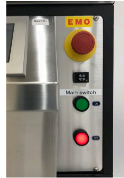
Figure 1: Emergency stop (EMO) and main ON/OFF switches
