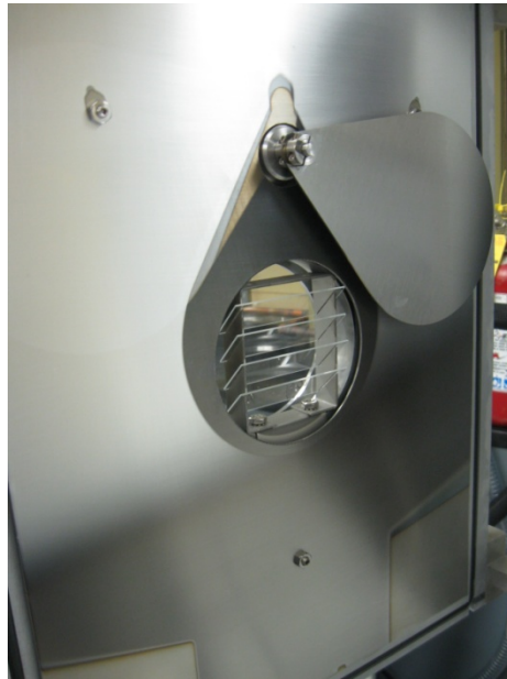
Figure 8: Change glass slides in the viewport as needed.
