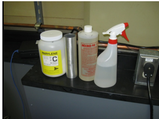
Figure 7: (L to R) Parylene C, boat form, concentrated Micro release agent, and 2% release agent.
