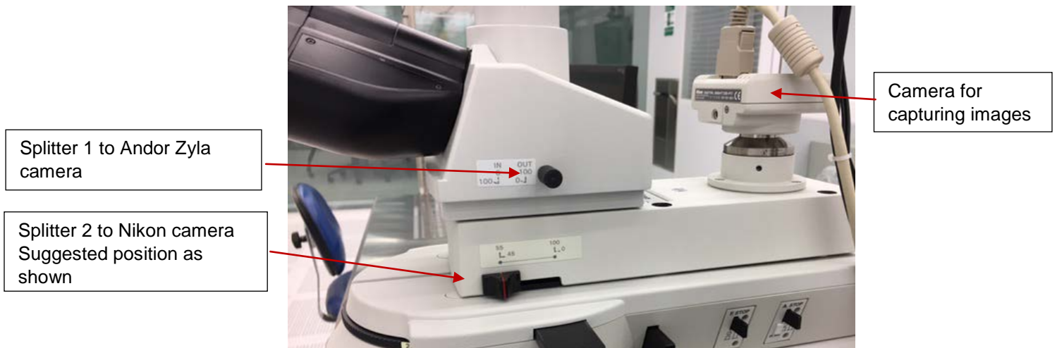
Figure 7. Observe using eyepiece and camera
