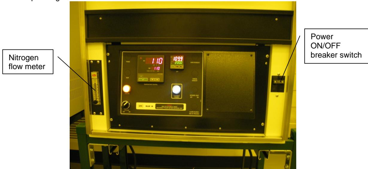
Figure 2: Front panel of the oven.
