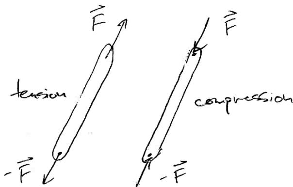
Observe that the *internal force* is uniform throughout the member and equal to force at the joint.
