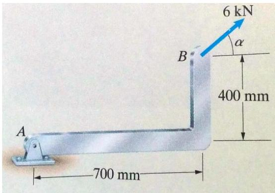
The L-shaped bar has a pin support at A and is loaded by a 6-kN force at B. Neglect the weight of the bar.
