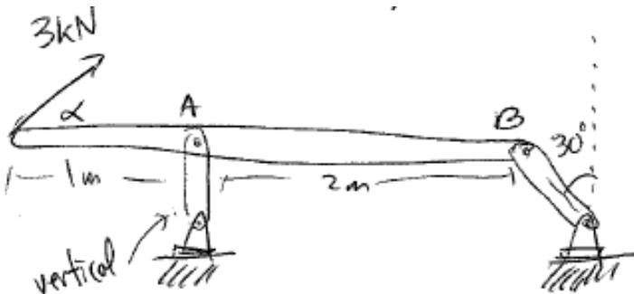
Determine the angle  $\alpha$  and the reactions at Points A and B.
