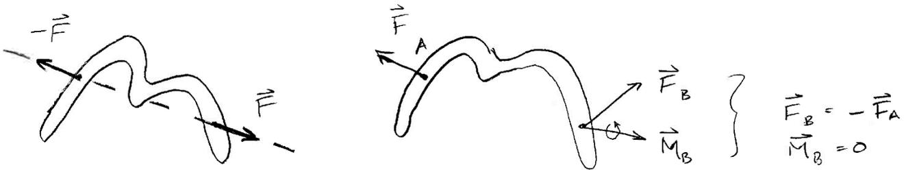
If an object is in equilibrium and subjected only to two forces<sup>3</sup>, or multiple forces that can be reduced to two equivalent forces, then the object is referred to as a two-force member, and the two forces
