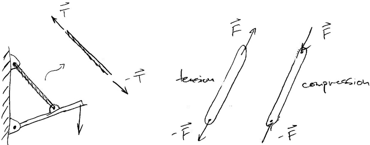
Example 5.11. Observe that we can already solve this problem, but go through it on your own to see how recognizing an object as a two-force member can simplify the solution<sup>4</sup>.
