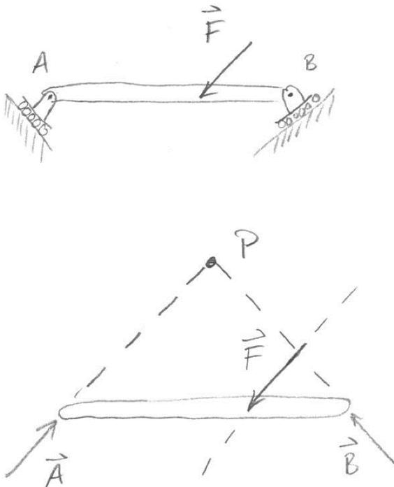
From the free-body diagram showing the lines of action, we see clearly that the beam may rotate.
