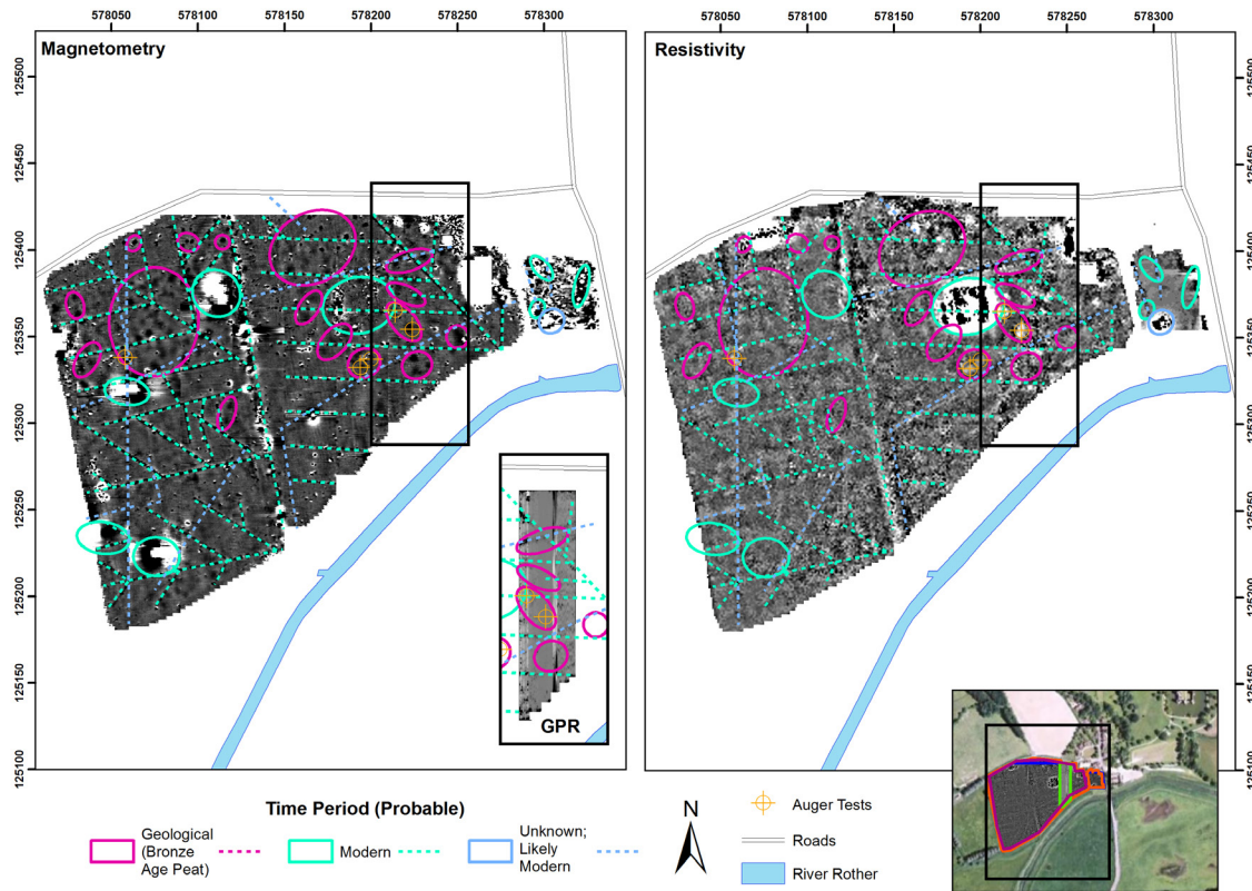
Fig. 4.13a: Cricket Field: Interpreted magnetometry, earth resistance, and GPR survey results. Large dipolar anomalies suggest large modern metallic deposits, while small dipoles could be modern debris, ancient peat, or any metallic deposit of intermediate age. Positive magnetic anomalies are likely Bronze Age peat deposits. The large resistance anomaly is the modern, maintained cricket pitch. Linear magnetic anomalies are almost certainly post-medieval or early modern drains; linear resistive anomalies are less certain. No evidence of a leat was observed.
