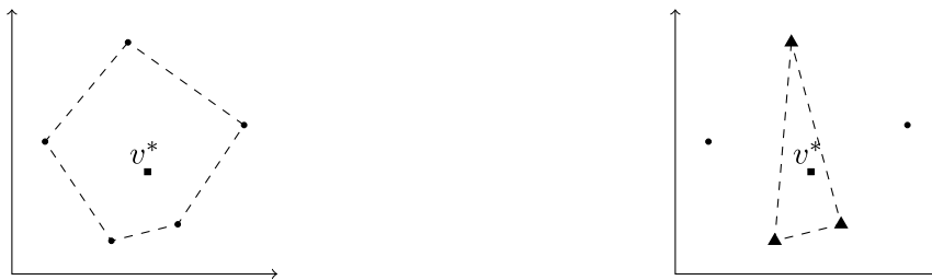
Fig. 1. In this example, n = 2 . In the left panel, the round dots are elements of V and the square is v^* . The dashed polytope depicts co(V) . In the right panel, the triangles are elements of V' , the round dots are elements of V \setminus V' and the square is v^* . The dashed polytope depicts co(V') . Since n = 2 , V' can be chosen such that \#V' \leq 3 .
