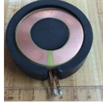
Fig. 10: Picture of the modified self-resonant structure that was used for experimental results.
