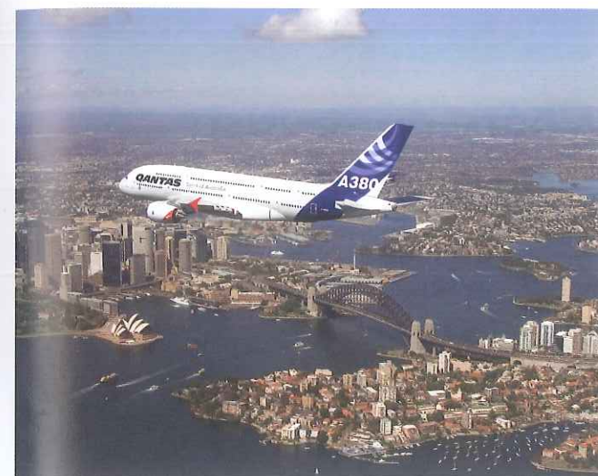
2.1.3 The Airbus 380 is the largest jet plane in the world. It is wide-bodied and double-decked, which enables it to carry large numbers of passengers—either 525 passengers in three classes, or 853 passengers all flying economy.
