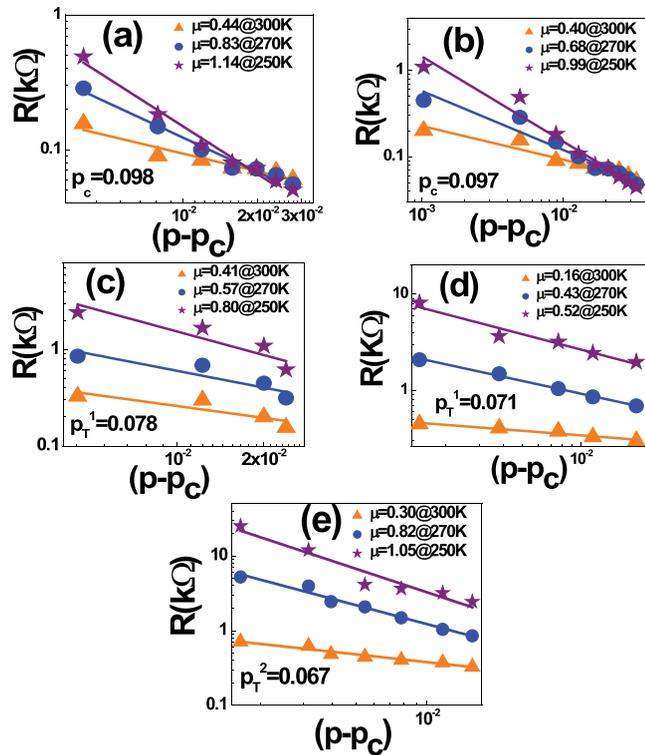
FIG. 4. Scaling behavior of the sample resistance near different percolation thresholds at temperatures 300 K, 270 K, and 250 K. Values of percolation thresholds determined in Fig. 3 are used, with the corresponding critical exponents indicated in each panel.
