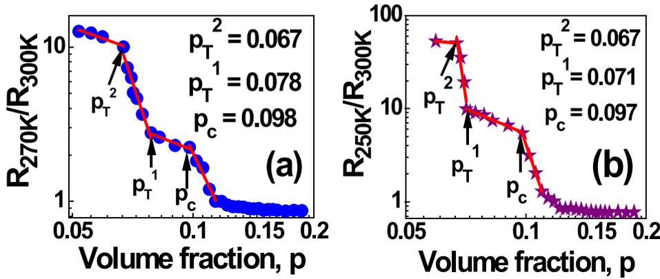
FIG. 3. Resistance ratios (a)  $R_{270K}/R_{300K}$  and (b)  $R_{250K}/R_{300K}$  as a function of volume fraction  $p$ . Three percolation thresholds,  $p_T^1$ ,  $p_T^2$  (first and second tunneling thresholds), and  $p_c$  (the classical percolation threshold), are identified from the inflection points of the power law fitting in the log-log plots.
