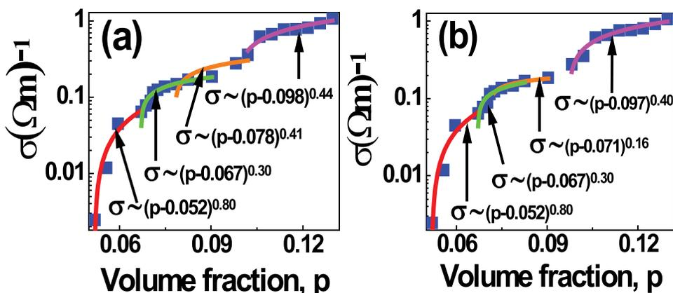
FIG. 2. System conductivity as a function of volume fraction of RuO<sub>2</sub>, as measured at 300 K. Two sets of slightly different percolation thresholds are used in the power law fitting, including: (a) thresholds found from the resistance ratio  $R_{270K}/R_{300K}$  measurement given in Fig. 3(a); and (b) thresholds extracted from the  $R_{250K}/R_{300K}$  measurement in Fig. 3(b).
