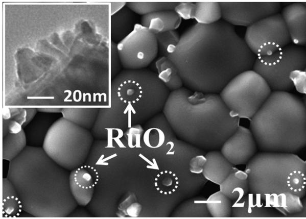
FIG. 1. SEM image of RuO<sub>2</sub>-CCTO composite system, with RuO<sub>2</sub> particles indicated by dotted circles. Inset: High-resolution TEM image of grain structure in CCTO.
